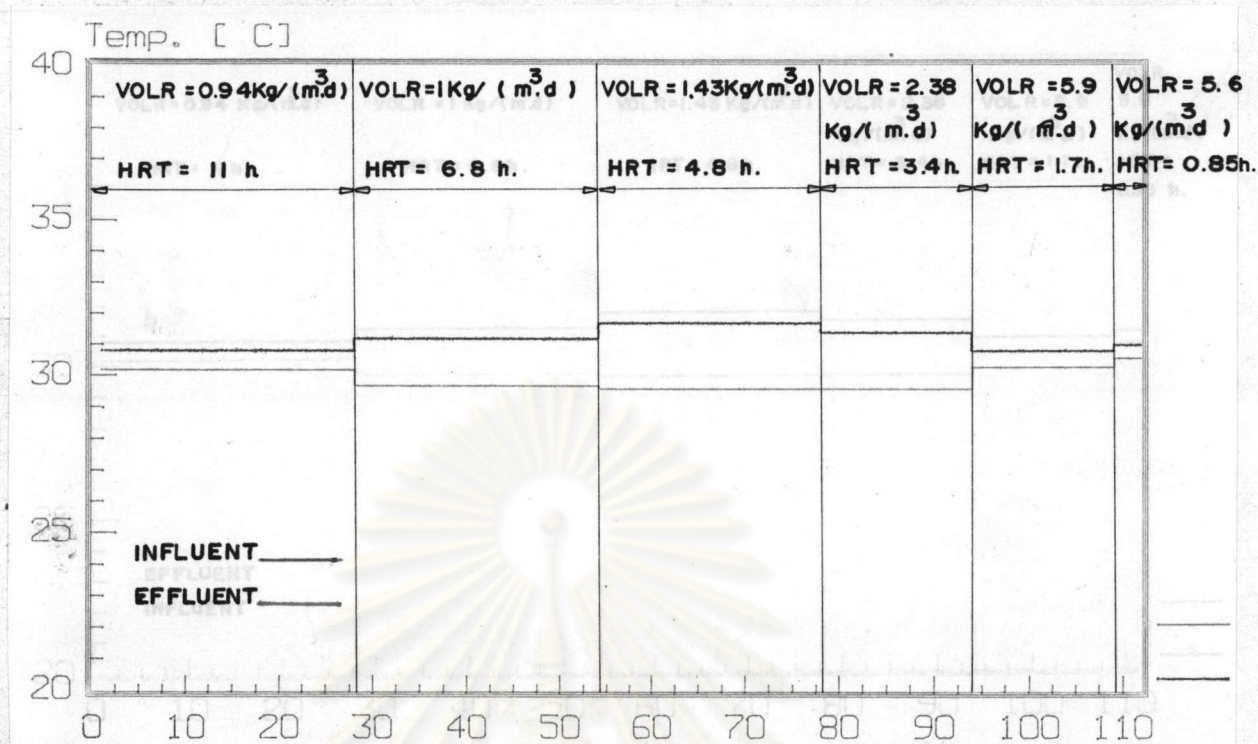
Figure 5.5.18 Average Influent and Effluent Temperature of Fixed Bed Reactor
