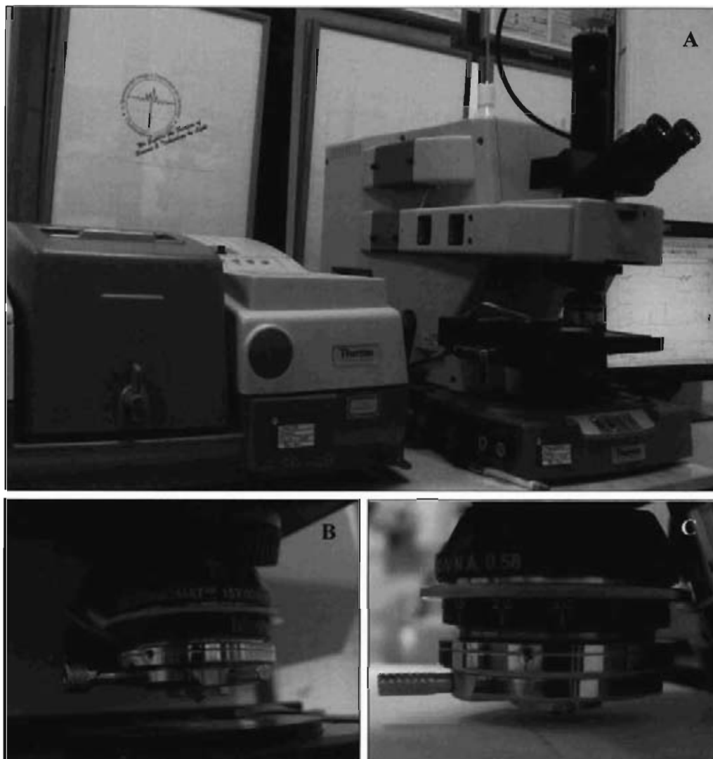
Figure 3.3 Example of procedures for spectral acquisition (A) Continuum infrared microscope attached to an infrared spectrometer, (B) slide-on Ge \mu IRE is fixed on the position of slide-on housing attached to the 15X Schwarzschild-Cassegrain infrared objective, and (C) the complete homemade \mu ATR accessory ready for a spectral acquisition.
