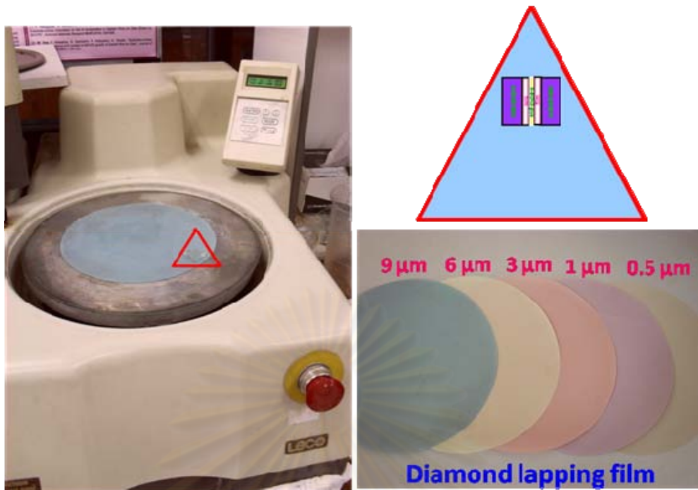
Figure 3.5: (left) The specimen is polished by the 9 \mu\text{m} diamond lapping film on the polisher, (right-top) Sample model of the clamped specimen is stuck on a triangular shaped glass and (right-below) showing the diamond grind size of diamond lapping films.
