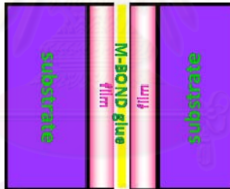
Figure 3.4: Sample model of the two pieces of specimen are stuck by M-BOND glue
