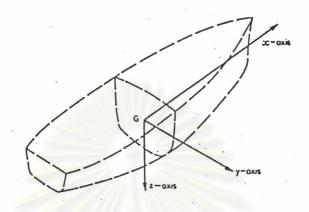
Fig. (2.1) Define ship's reference axes
