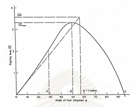
Fig. (2.13) Curve of statical stability
