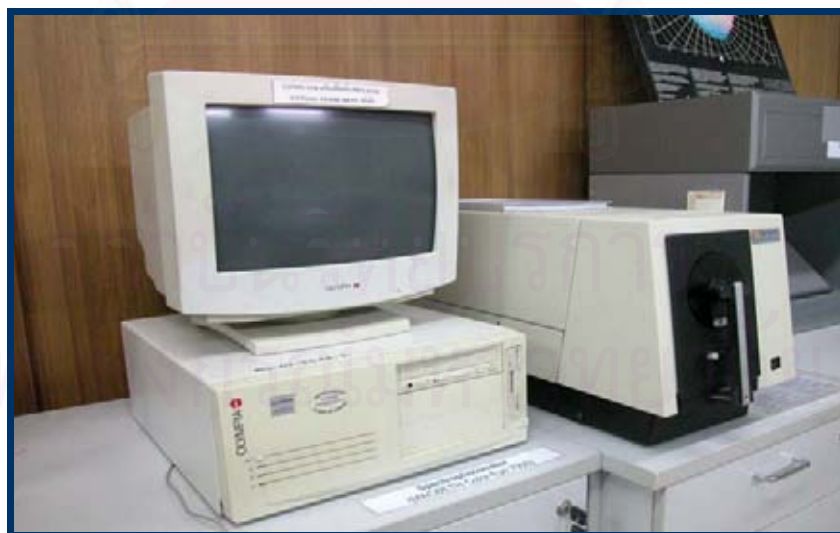
Figure 3.12 Spectrophotometer (Macbeth ColorEye 7000)
