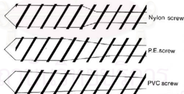
Figure 2.5 Variations in screw design
