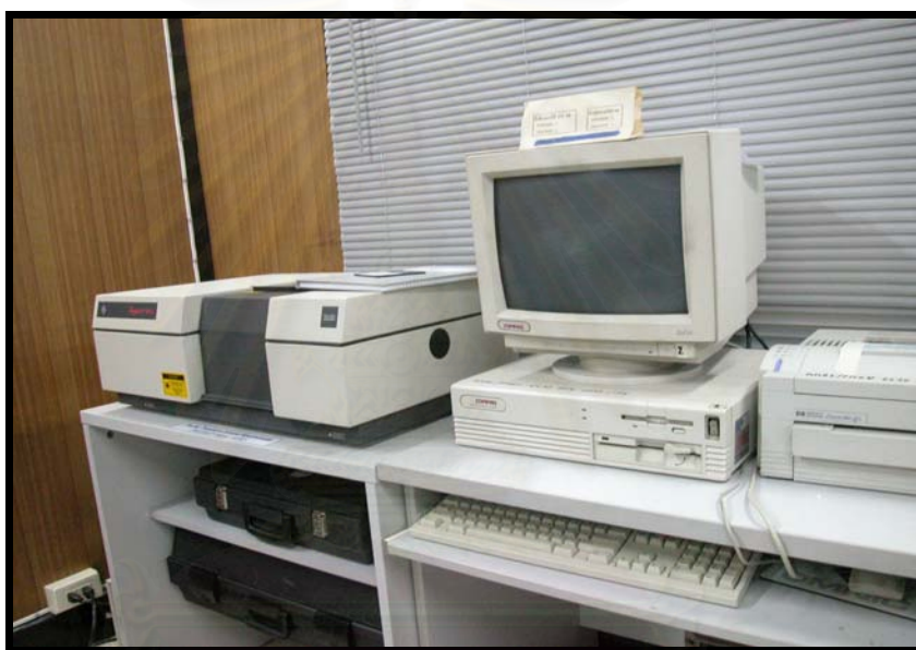
Figure 3.9 Fourier Transform Infrared Spectroscopy (Nicolet Impact 400D)
