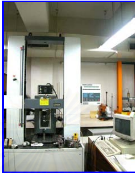
Figure 3.11 Universal testing machine (Lloyd LR100K)
