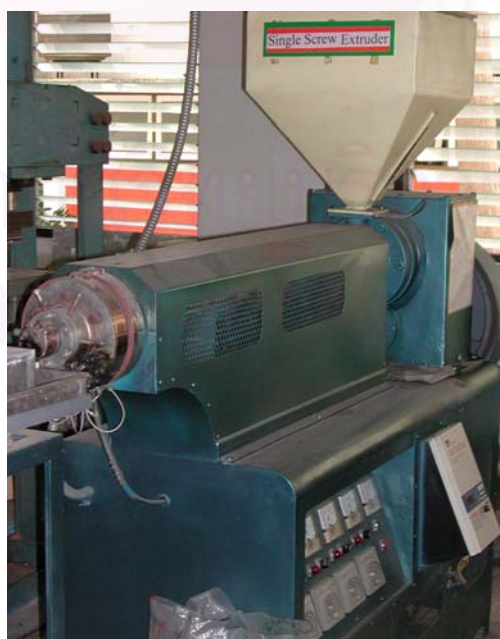
Figure 3.3 Single screw extruder (Powtran Invada 9308)
