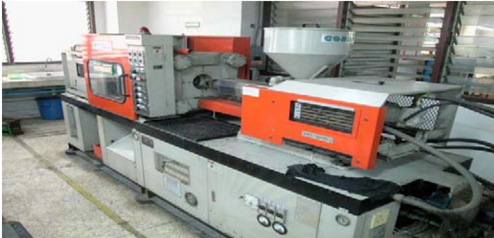
Figure 3.5 Injection molding machine (Cosmo)
