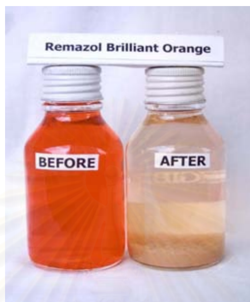
Figure 5.5. Characteristics of synthetic wastewater containing of Remazol Brilliant Orange 3R before and after batch decolorization by the mixed culture of strain S1 and A5
