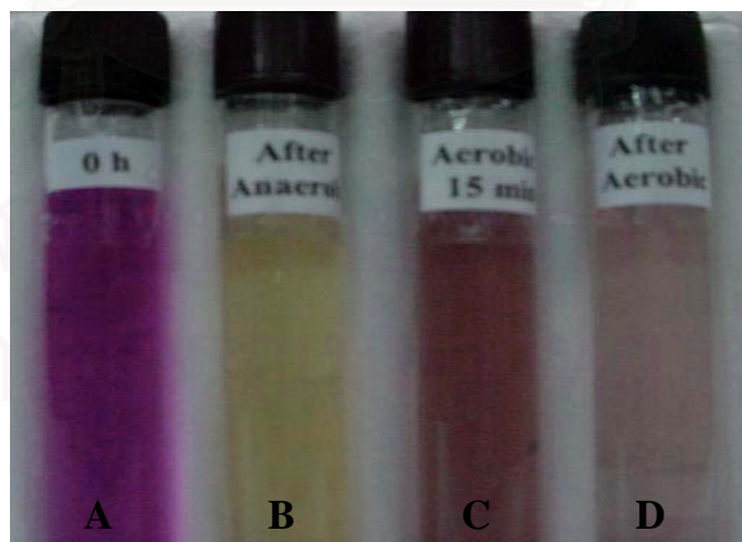
Figure 8.15 Characteristics of synthetic textile wastewater containing Remazol Brilliant Violet 5R at (A) the beginning of anaerobic phase, (B) after anaerobic phase (C) 15 min after aerobic phase and (D) after aerobic phase
