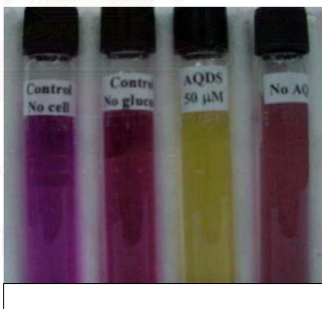
Figure 7.16 Reduction of Remazol Brilliant Violet 5R by Paenibacillus sp. strain A5 on mineral medium containing glucose in the presence and absence of AQDS. (A) Control without cells (B) control without glucose (C) cells plus AQDS and glucose (D) cells plus glucose without AQDS
