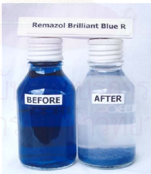
Figure. 5.27 Characteristics of synthetic textile wastewater containing of Remazol Brilliant Blue R before and after batch decolorization by the mixed culture of strain S1 and A5
