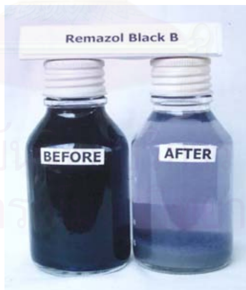
Figure. 5.12 Characteristics of synthetic textile wastewater containing of Remazol Black B before and after batch decolorization by the mixed culture of strain S1 and A5
