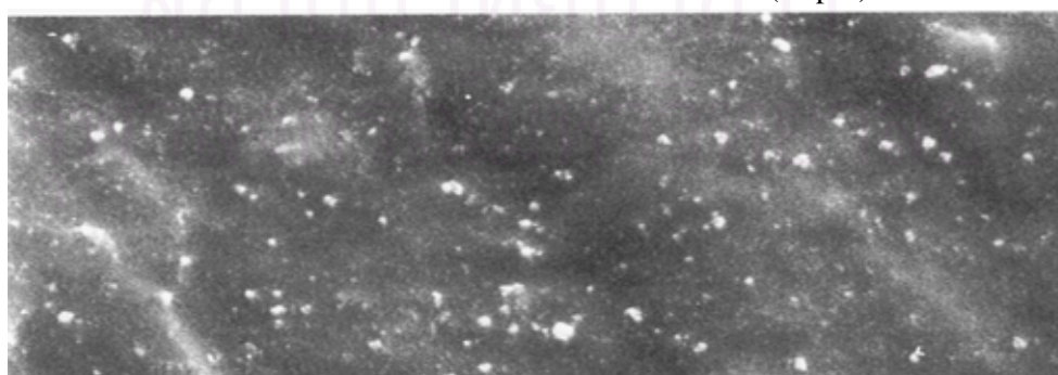
NBR with in situ silica from E PS (35 phr)
