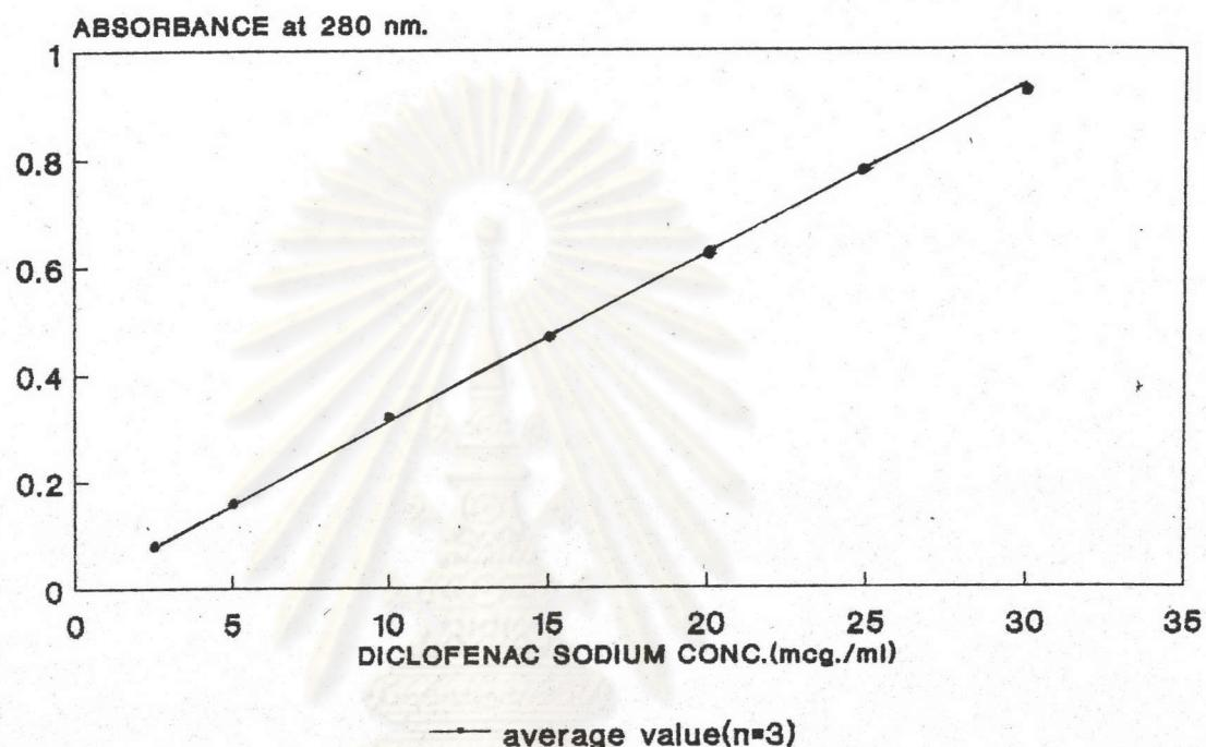
Figure 18 Calibration curve of diclofenac sodium in simulated intestinal fluid T.S. without enzyme (pH 7.5  $\pm$  0.1)
