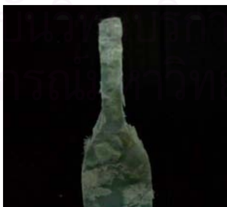
Figure 4.9 A sample of filled HDPE after subjecting to tensile test
