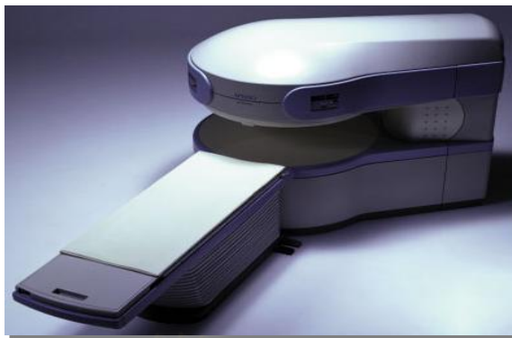
Figure 2.3 Open MRI magnet (Aperto presentation, Hitachi Company)
