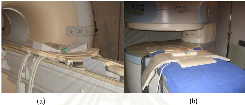
Figure 3.8 The experimental set up of duct phantom for evaluation of spatial resolution, SNR and CNR at MRI 3.0 T (a) and 0.4 T (b).
