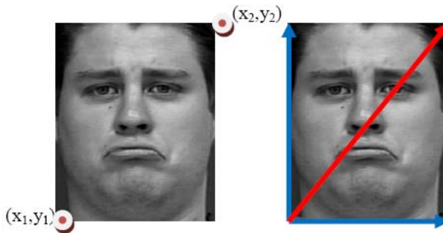
Figure 4.2: Normalized distance by dividing original distance with diagonal line across the face
