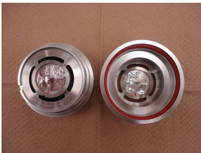
Figure 4-8 Illustration of detector channel at each impactor plate geometry.
