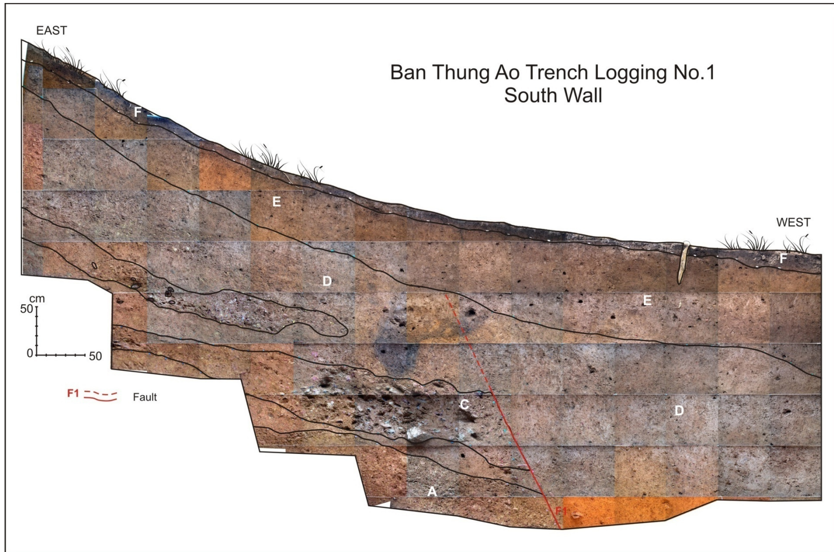
Figure 4.28 View of paleoseismic trench section (no.1) on the south wall, Ban Thung Ao village, Nan, showing Quaternary stratigraphy and fault orientation.
