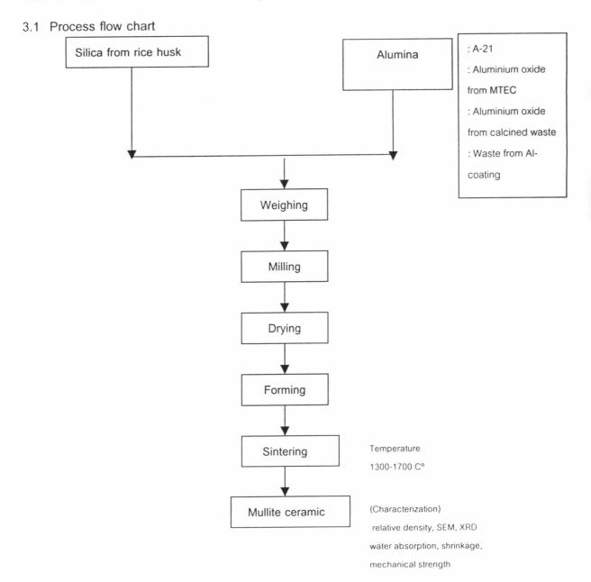
Fig.3.1 Flow chart for the synthesis of mullite
