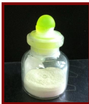
Figure A.1 Ni/CaO (multifunctional catalyst in powder form) used for hydrogen production by sorption enhanced steam methane reforming process
