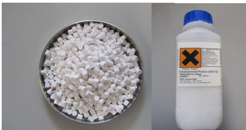
Figure A.2 Hydrotalcite sorbent (pellet form) used in CO 2 adsorption experiment for the data in the simulation
