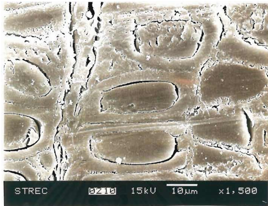
Figure 4.15 SEM micrograph of transverse section of polymer filled cells (1500x)
