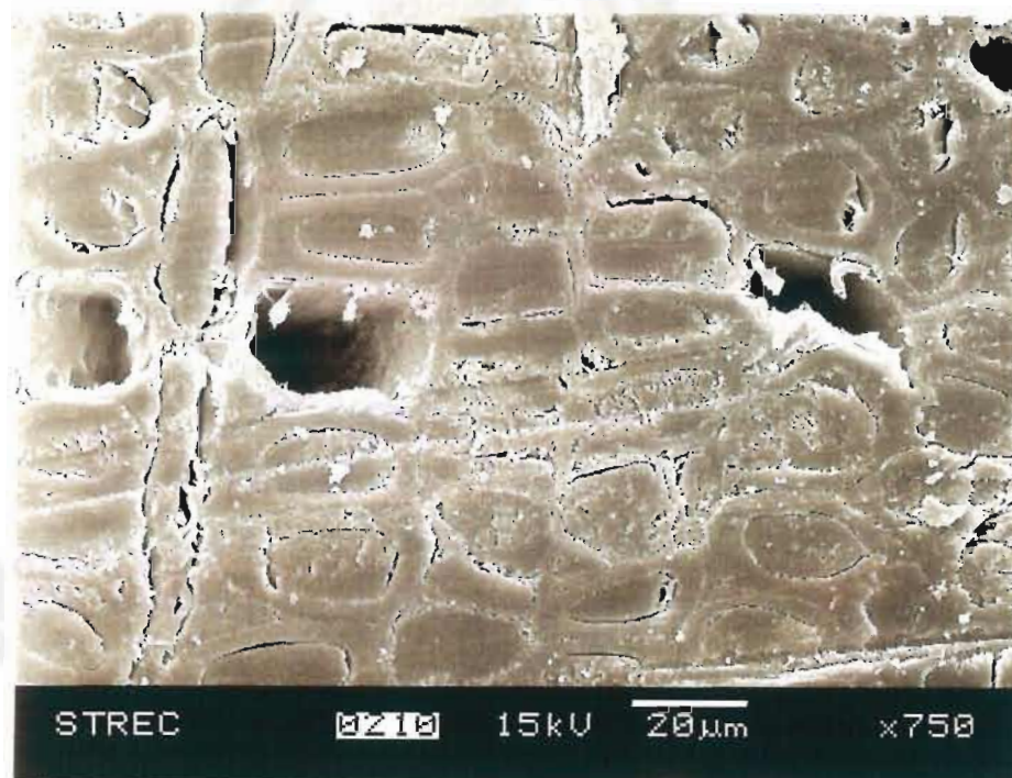
Figure 4.14 SEM micrograph of transverse section of polymer filled cells (750x)
