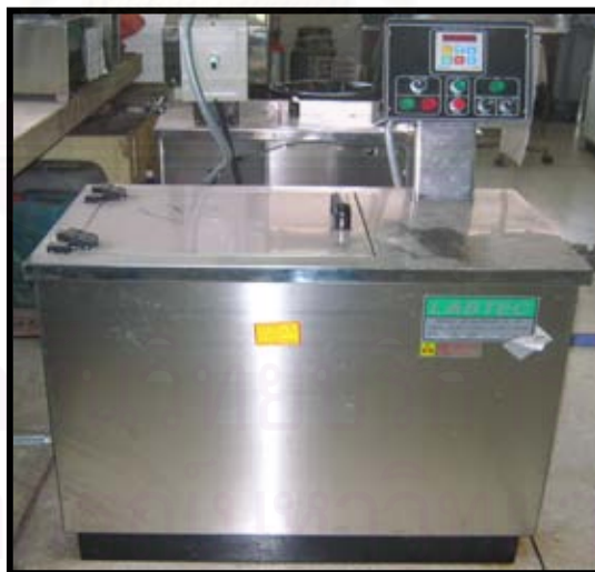
Figure 3.8 Laboratory exhausted dyeing machine, Labtec®
