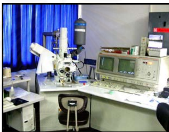
Figure 3.5 Scanning electron microscope (JSM-6400)
