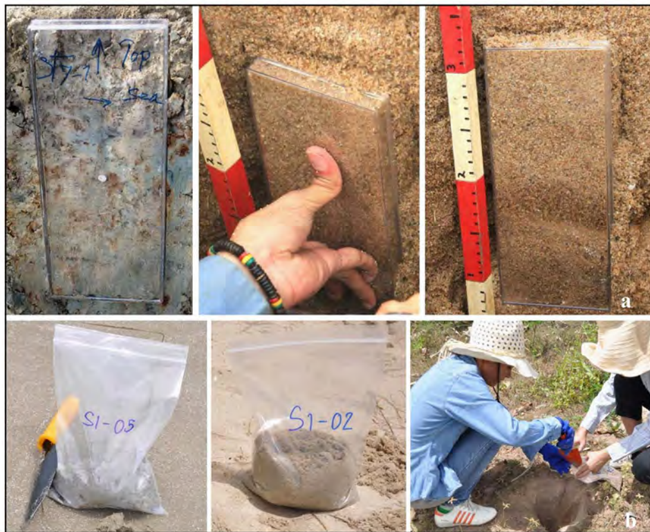
Figure 3.4 Lunch box a) and bulk sample b) technique using in this study.
