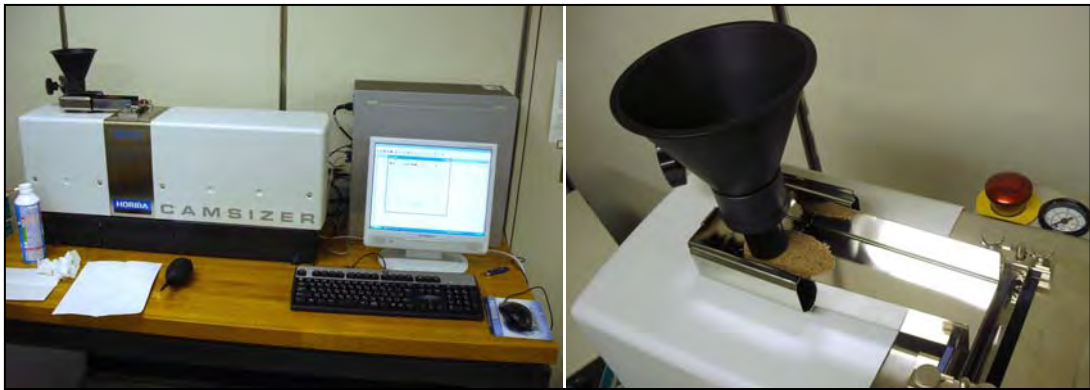
Figure 3.7 Camsizer, a particle analysis by digital image processing method, at GSJ using in this study.
