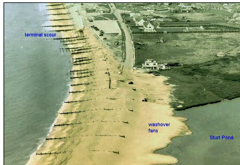
Figure 2.1 Oblique photo showing washover sediments penetrated into a pond at the coastline of Hurst Spit, Milford on Sea, Southern England in 1958. ( http://www.soton.ac.uk/~imw/jpg-Hurst/6HS-1958-Milford.jpg )
