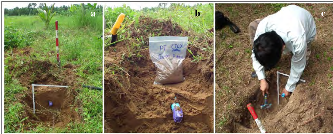
Figure 4.15 a) Pictures showing small pit for collecting sediment samples for TL dating. b) Annual dose in plastic bag and paleo dose in opaque plastic tube. c) Sediment sampling by opaque plastic tube for paleo dose. Pictures taken locations are refer to the 2 nd and 3 rd ridge in Figure 4.13.
