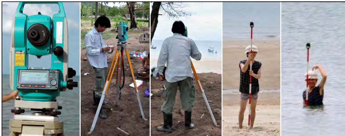
Figure 3.6 Digital survey camera using for beach profile measurement at the coastal area.
