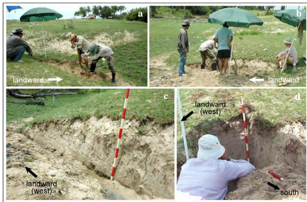
Figure 4.37 a) and b) Trenching perpendicular to the shoreline at the margin of washover terrace. c) Washover successions at the avalanche face thick 80 cm. d) Trenching in west and south direction for observing 3D sedimentary structure. Pictures taken location refer to Figure 4.35.
