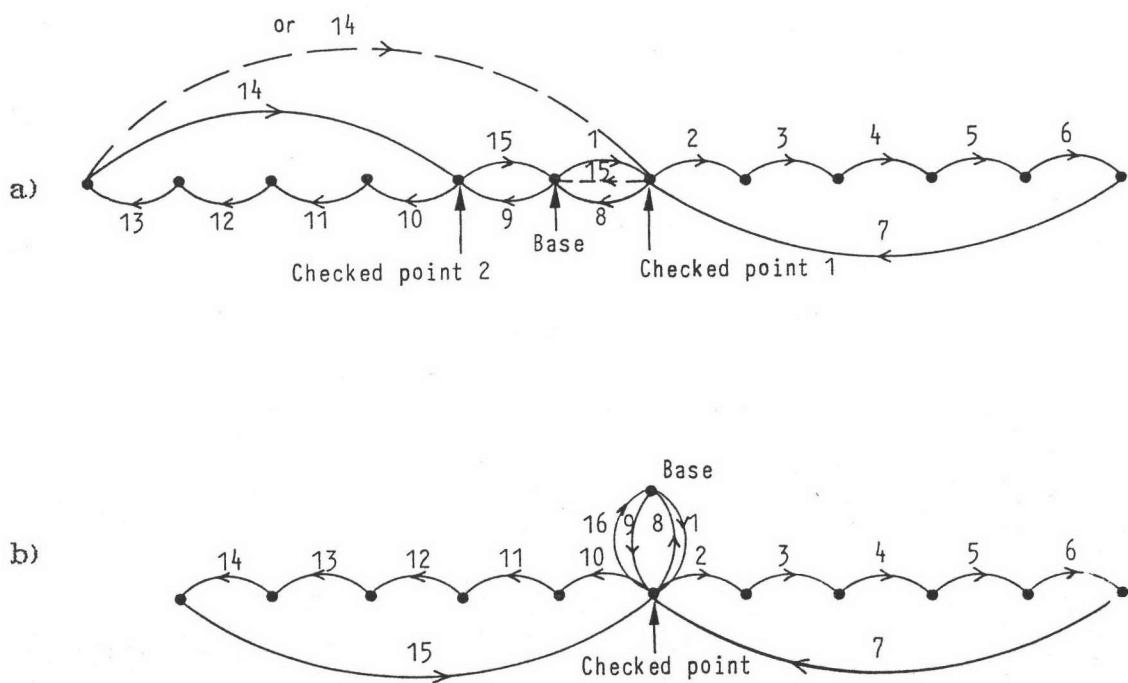
Figure B2 Sequence of looping gravity meter observations; a) type 1, base station is on observation line; b) type 2, base station is outside observation line.
