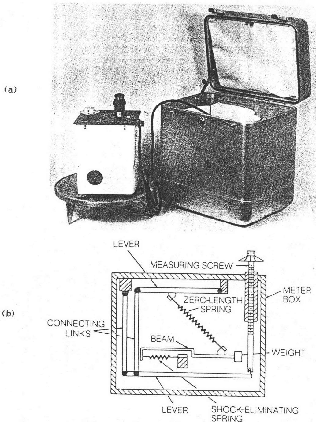
Figure B1 Showing photograph of the LaCoste-Romberg G series Gravimeter (a), and cross section (b) (after Robinson and Coruh, 1988).
