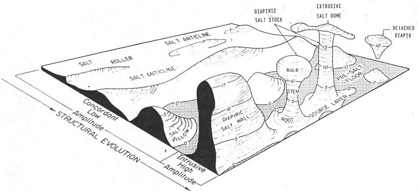
Figure B5 Shallow salt dome model diapiric salt stock and extusive salt dome
