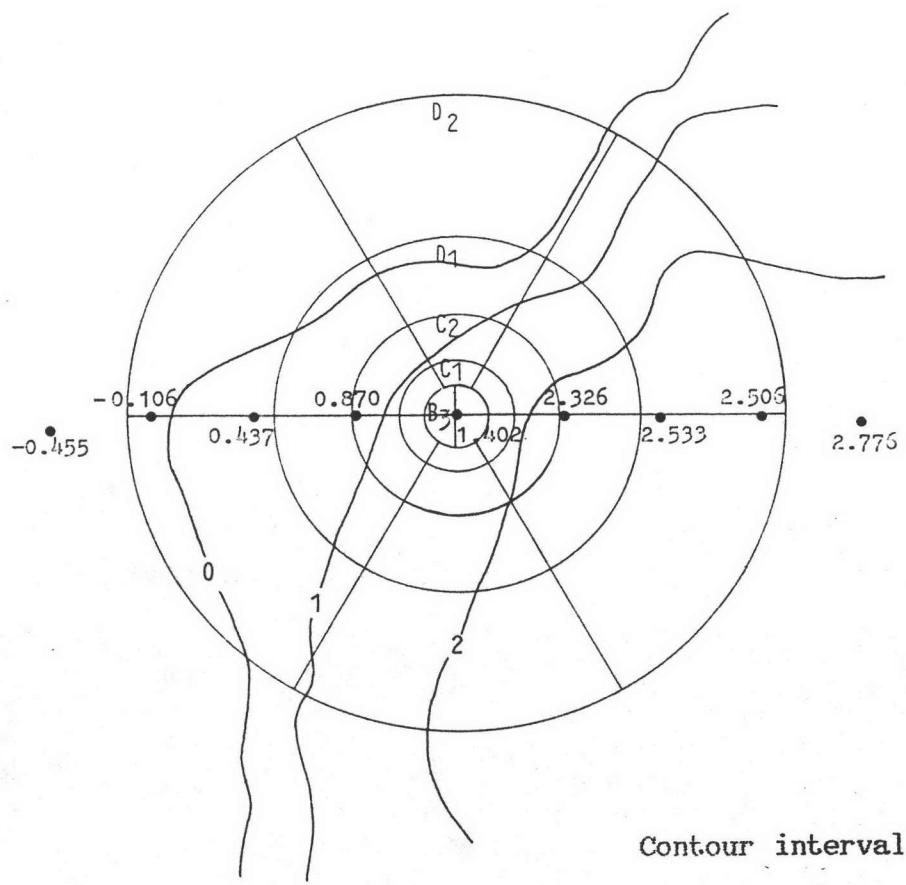
Figure B4 Use of terrain chart with topographic map (modified after Telford et al., 1983).
