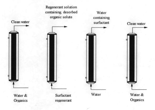
Figure 1.1 Process strategy for surfactant-enhanced carbon regeneration.
