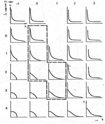
Figure 21 Matrix of speed-density relationships for various m, 1 combinations of the general car-following equation. (Dashed lines enclose limiting values of 1 and m used in Table 8)
