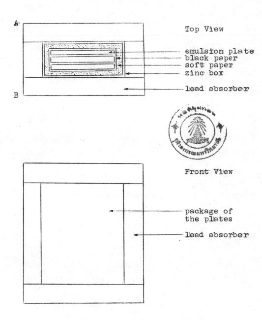
Fig I. The arrangement of the plates and absorber.
