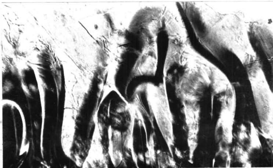
Fig.21 A 150\ \mu\text{m} -thick layer of EPAPV in an a.c. electric field of 6.4 \times 10^2 volts/cm at 90.6^\circ\text{C} with the free-lead electrodes having separation of 1.18\ \text{mm} .
