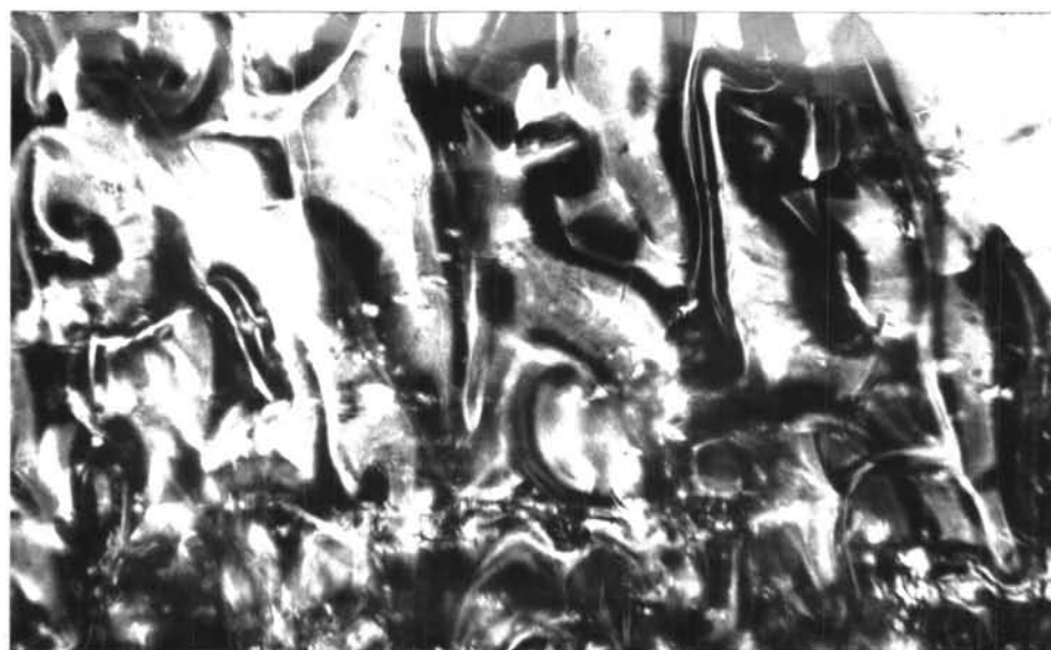
Fig.23 A 150 μm-thick layer of EPAPV in a d.c. electric field of 6.4 \times 10^2 volts/cm at 92.0 °C with the free-lead electrodes having separation of 1.18 mm.
