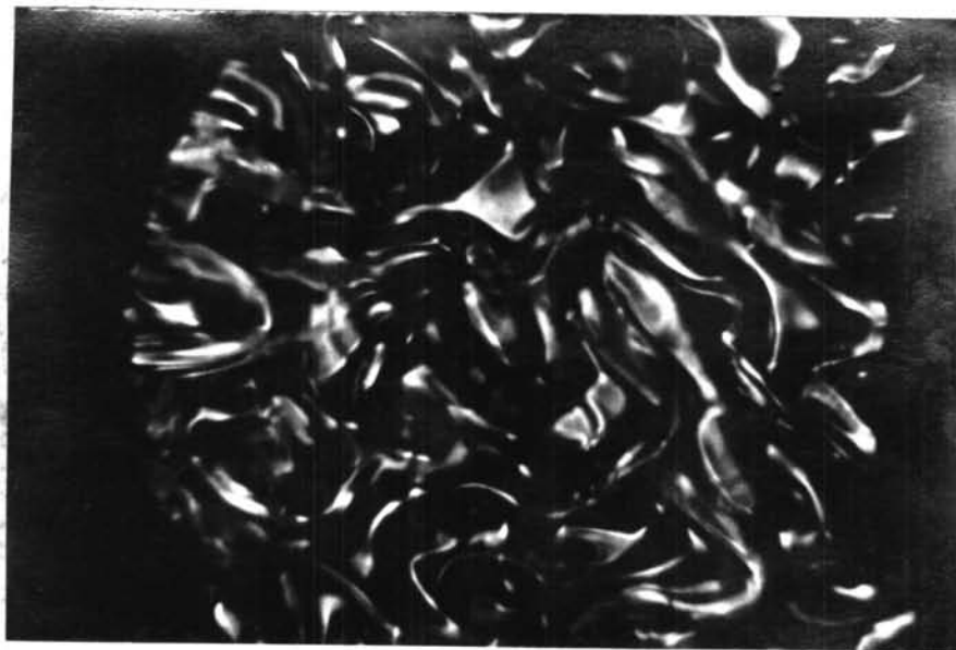
Fig.9 A 80\ \mu\text{m} -thick layer of EPAPV placed between transparent electrodes in an a.c. electric field of 3.8 \times 10^3 volts/cm at 81.2\ ^\circ\text{C} .
