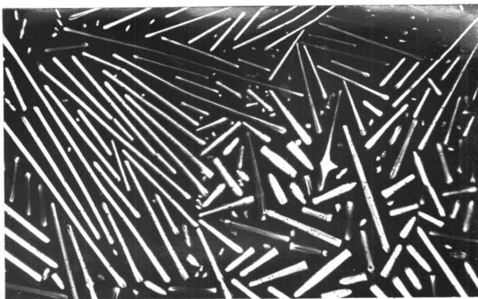
Fig.32 A 100 \mu\text{m} -thick layer of PCBAV placed between transparent electrodes in an a.c. electric field of 5.0 \times 10^3 volts/cm at 104.1^\circ\text{C} .
