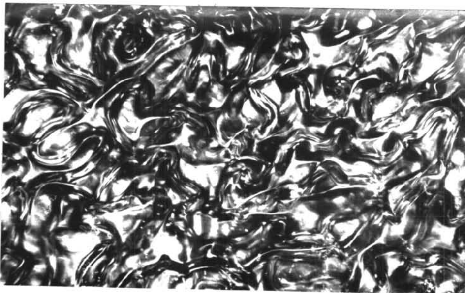
Fig.17 A 100 μm-thick layer of EPPHP placed between transparent electrodes in a d.c. electric field of 2.5 \times 10^4 volts/cm at 67.1 °C.
