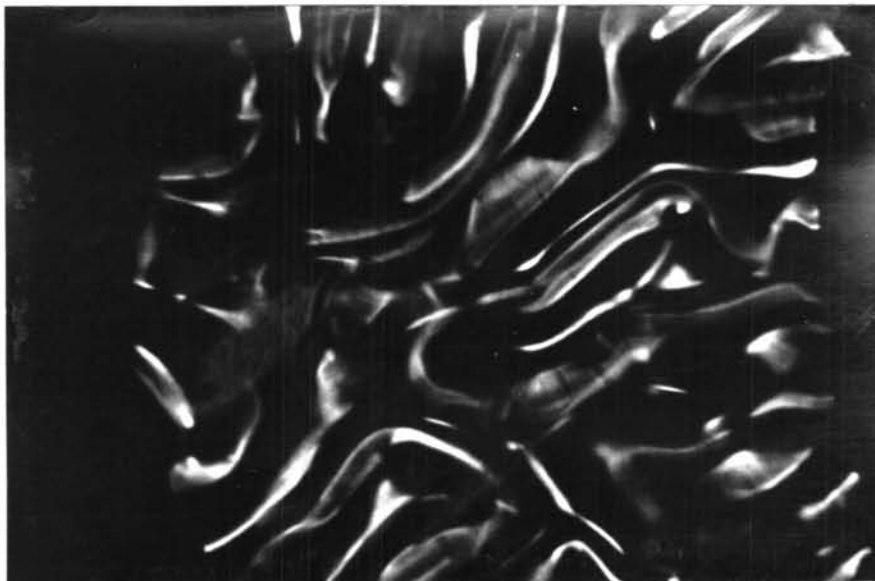
Fig.8 A 80\ \mu\text{m} -thick layer of EPAPV placed between transparent electrodes in an a.c. electric field of 2.5 \times 10^3 volts/cm at 97.5\ ^\circ\text{C} .
