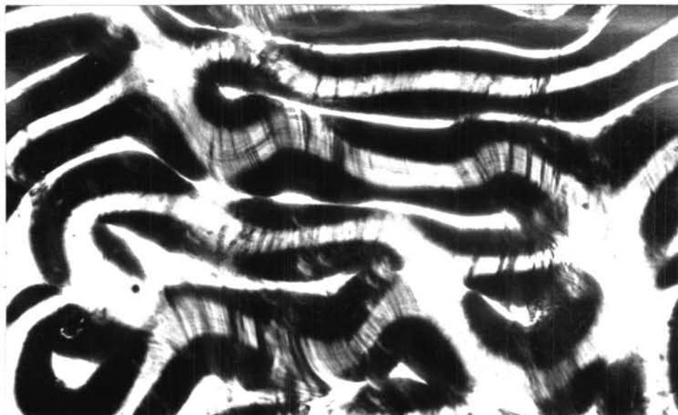
Fig.15 A 100 \mu\text{m} -thick layer of EPPHP placed between transparent electrodes in an a.c. electric field of 7.5 \times 10^3 volts/cm at 67.1^\circ\text{C} .
