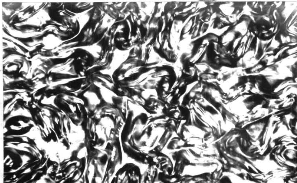
Fig.14 A 100 \mu\text{m} -thick layer of EPPHP placed between transparent electrodes in a d.c. electric field of 1.0 \times 10^4 volts/cm at 66.6^\circ\text{C} .
