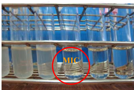
Figure 4.3 MIC of imipenem against one strain of P. aeruginosa was determined by broth macrodilution method.
