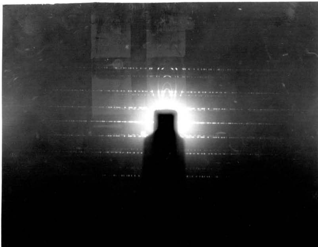
Fig. 4.2 Rotation photographs of Latifolin ( C_{17}H_{18}O_4 ) (a) 100 Rotation axis; CuK -radiation. (b) 010 Rotation axis; CuK -radiation.
