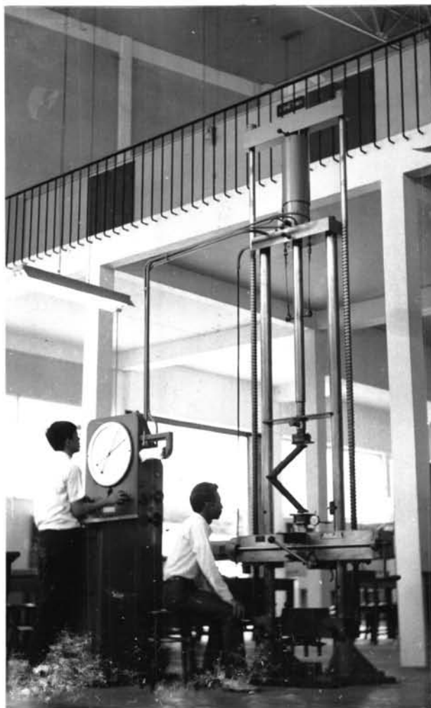
Fig. A35. PIPE BEND UNDER IN-PLANE BENDING LOAD OF AMSLER TESTING MACHINE.
