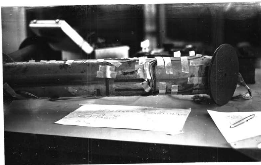
Fig. A42. GAGE POSITIONS FOR THE MEASURING OF LONGITUDINAL AND CIRCUMFERENTIAL STRAINS.
