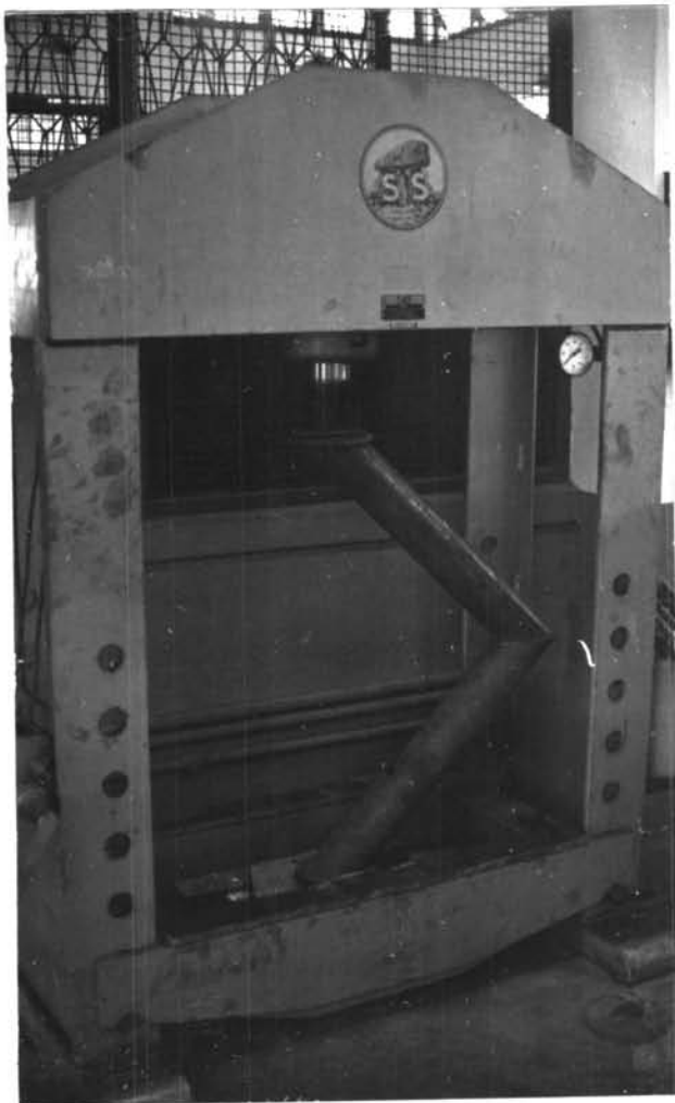
Fig. A37. PIPE BEND UNDER IN-PLANE BENDING LOAD OF SIGURD STENHØJ TESTING MACHINE.
