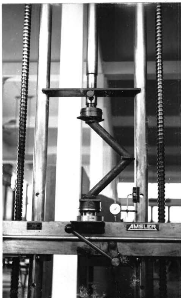
Fig. A36. PIPE BEND UNDER IN-PLANE BENDING LOAD OF AMSLER TESTING MACHINE.
