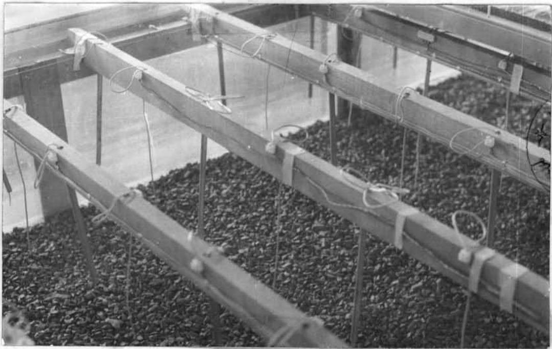
FIGURE 4.9 THERMOCOUPLES MOUNTED IN THE BASIN
