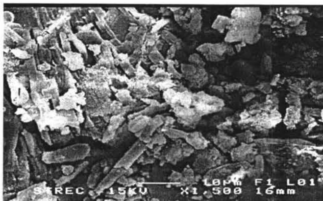
Figure C2 Micrographs of polystyrene polymerized in 10%wt CTAT, 1.6 mole of CTAT: 1 mole of styrene and 15 mole of styrene:1 mole of AIBN at 70 °C with 1500X magnification.
