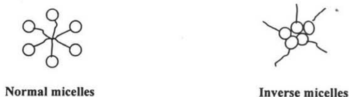
Figure 2.9 Schematic diagram of normal micelles and inverse micelles.
