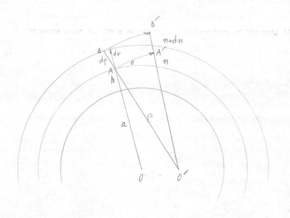
Fig. 1 Differential geometry used in the derivation of the effective-earth's radius model atmosphere.
