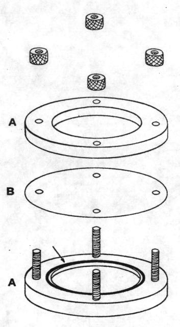
Figure 1 Diffusion cell used for release experiments.
