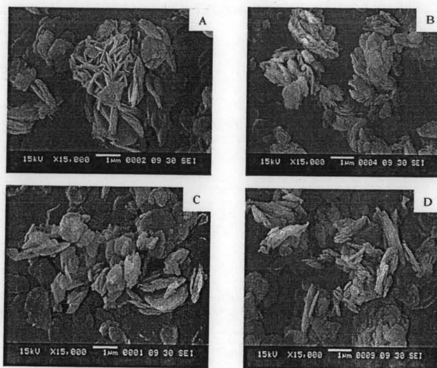
Figure 4.4 SEM images of calcined sample (A) Na-MCM-22(30), (B) H-MCM-22(30), (c) H-MCM-22(60) and (d) H-MCM-22(120) catalysts.
