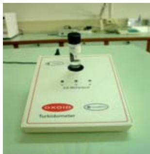
Figure 9 Turbidometer (McFarland) : use for measuring density of VRE suspension in MIC methods.
