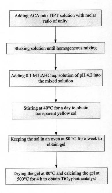
Figure 3.1 Preparation procedure for synthesized mesoporous TiO<sub>2</sub> photocatalyst.
