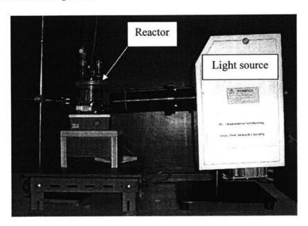
Figure 3.3 Setup of photocatalytic H<sub>2</sub> evolution system.
