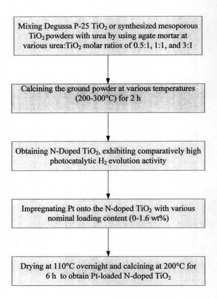
Figure 3.2 Preparation procedure for N-doped TiO<sub>2</sub> and Pt-loaded N-doped TiO<sub>2</sub> photocatalysts.
