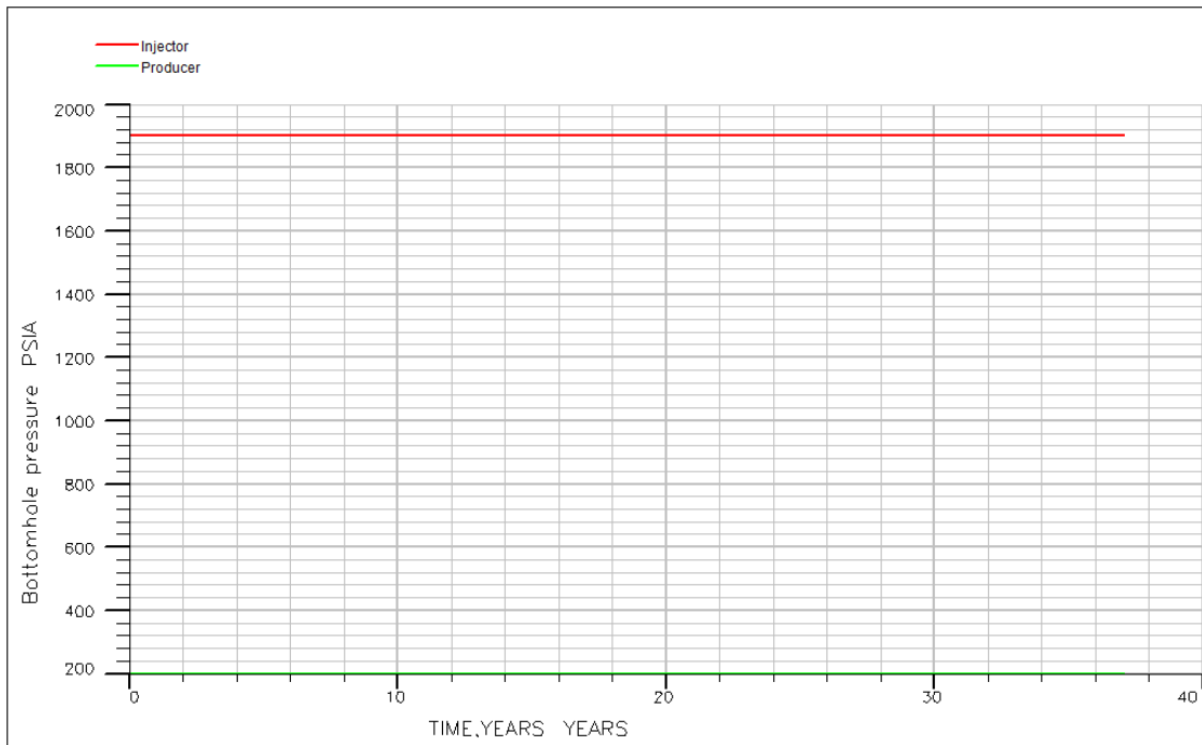
Figure 5.22 Bottomhole pressures of injector and producer of the case 0.10 PV pre-flushed water slug size followed polymer slug size as functions of time
