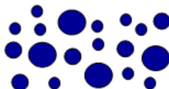
Figure 2.7 Broader distribution of polymer polyol particles can reduce viscosity
