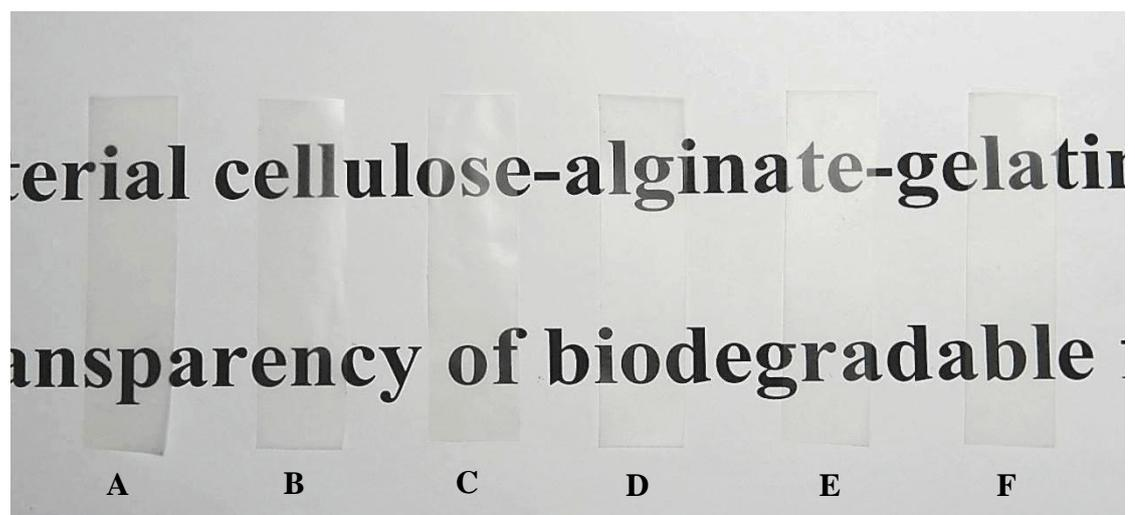
**Figure 4.2** Transparency of films: the BAG films at a ratio of 60/10/30 (A), 60/20/20 (B) and 60/30/10 (C), and the MBAG films at a ratio of 60/20/20 with glycerol (D), sorbitol (E), the mixture of glycerol and sorbitol (F)
