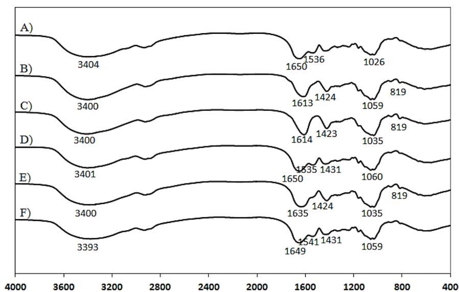
**Figure 4.4** FT-IR of BAG films at a ratio of 60/10/30 (A), 60/20/20 (B), 60/30/10 (C) and films at a ratio of 60/20/20 with glycerol (D), sorbitol (E) and the mixture of glycerol and sorbitol (F) addition, respectively.
