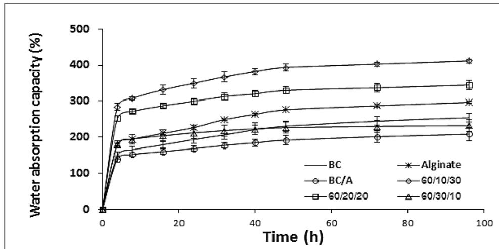
**Figure 4.5** Water absorption capacity (%) of the composite films: BC (—); Alginate (—\*—); BC/A (—○—); BAG films at a ratio of 60/10/30 (—◇—), 60/20/20 (—□—) and 60/30/10 (—△—) without plasticizer, respectively.
