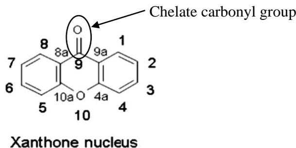
**Figure 4.25** Chelating of carbonyl group in the backbone of xanthone (Chaverri et al., 2008)
