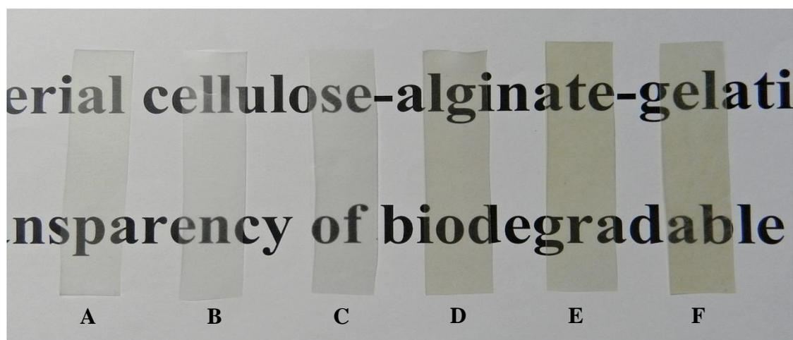
**Figure 4.22** Transparency of films: the BAG films at a ratio of 60/20/20 without plasticizer (A), with glycerol (B), with glycerol and adding tannic acid at a ratio of 10 mg (C) tannic acid per g gelatin solution, with glycerol, tannic acid and the mangosteen ethanolic extract at concentration of 1% (D), 5% (E) and 10% (F) v/v, respectively.
