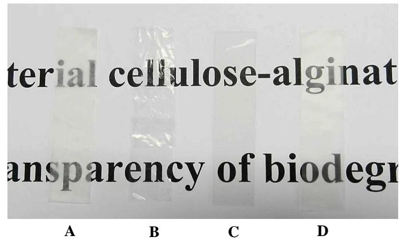
**Figure 4.1** Transparency of films: bacterial cellulose (A), sodium alginate (B), gelatin (C) and BC/A at a ratio of 60/40 (D)
