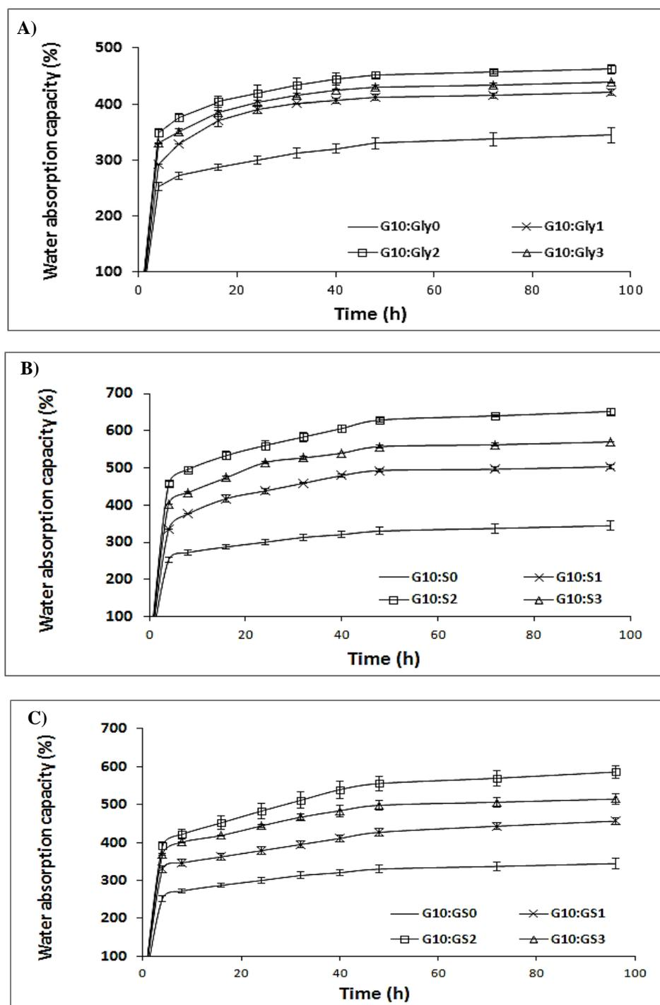
**Figure 4.6** Water absorption capacity (%) of the composite films: films at a ratio of 60/20/20 with glycerol (A), sorbitol (B) and the mixture of glycerol and sorbitol (C); G:Gly, G:S and G:GS refer to a ratio of gelatin to glycerol, sorbitol and the mixture of glycerol and sorbitol (w/w), respectively.
