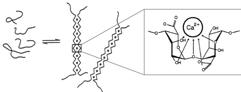
**Figure 2.6** Schematic representation of the egg-box association of the poly-L-gulonate sequences of alginate crosslinked by calcium ions. The figure shows conversion of random coils to buckled ribbon like structures which contain arrays of Ca<sup>2+</sup> ions. The magnified figure shows the proposed stereochemistry of Ca<sup>2+</sup> ion complexation. The oxygen atoms involved in the coordination sphere are shown as filled circles (Rees, 1981, modified).
