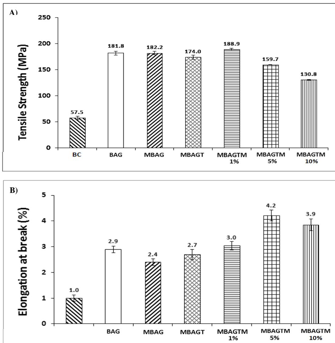
**Figure 4.27** Mechanical properties of MBAGTM films in dry state at 1%, 5% and 10% v/v concentration of mangosteen ethanolic extract: Tensile strength (A) and Elongation at break (B).
