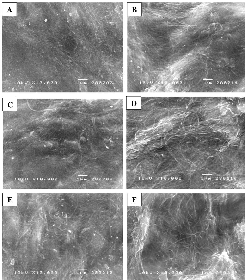
**Figure 4.20** SEM images of surface morphology of MBAGT films in dry (left) and re-swollen (right) forms at a ratio of mg tannic acid to gram gelatin solution at 5 mg (A and B), 10 mg (C and D) and 15 mg (E and F).
