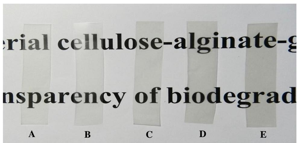
**Figure 4.14** Transparency of films: the BAG films at a ratio of 60/20/20 without plasticizer (A), with glycerol (B), with glycerol and adding tannic acid at a ratio of 5 mg (C), 10 mg (D) and 15 mg (E) tannic acid per g gelatin solution, respectively
