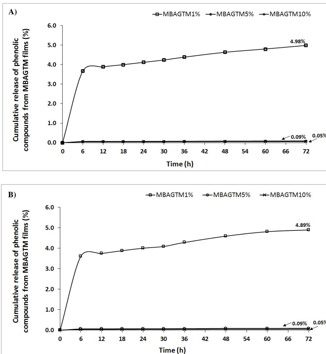
**Figure 4.35** Cumulative release profile of phenolic compound from MBAGTM films in acetate buffer at pH 5.6 (A) and PBS at pH 7.4 (B) reported as the percentage of the weight of phenolic compound (GAE) released divided by the actual amount of phenolic compound; MBAGTM at 1% ( $\square$ ), 5% ( $\circ$ ) and 10% ( $\times$ ) v/v, respectively
