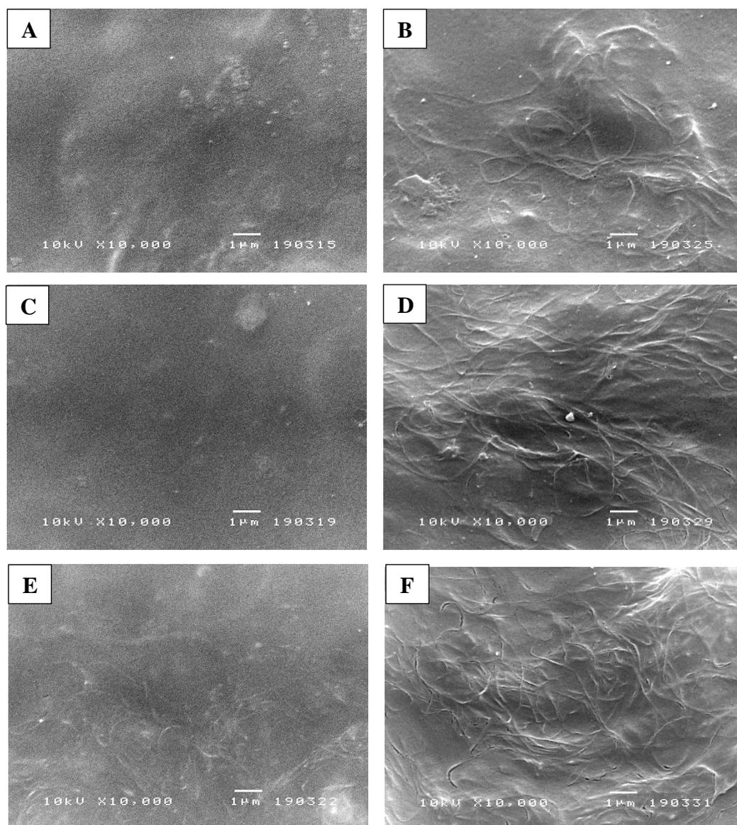
**Figure 4.30** SEM images of surface morphology of MBAGTM films in dry (left) and re-swollen (right) forms at concentration of 1% (A and B), 5% (C and D) and 10% (E and F) v/v mangosteen ethanolic extract.
