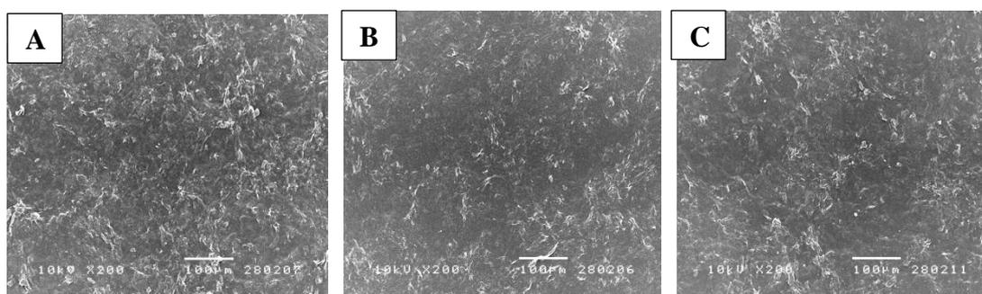
**Figure 4.19** SEM images of overview surface morphology of MBAGT films in dry form at ratio of mg tannic acid to g gelatin solution (w/w): 5 mg (A); 10 mg (B); 15 mg (C).
