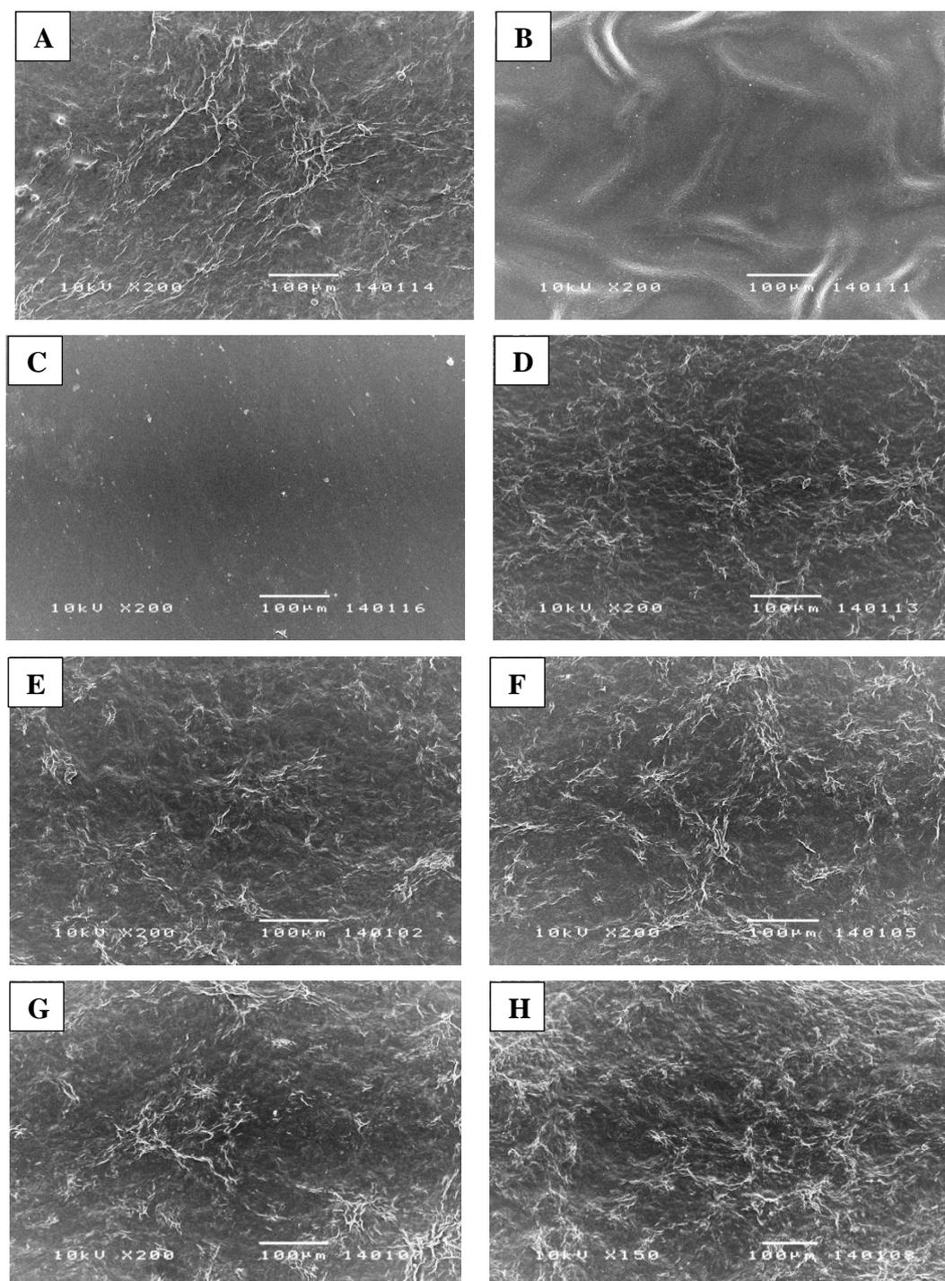
**Figure 4.11** SEM images of overview surface morphology of the films in dry state: BC (A); Sodium alginate (B); Gelatin (C); BC/A (D); BAG films at a ratio of 60/10/30 (E), 60/20/20 (F), 60/30/10 (G) and MBAG film at a ratio of 60/20/20 plasticized with glycerol (H).
