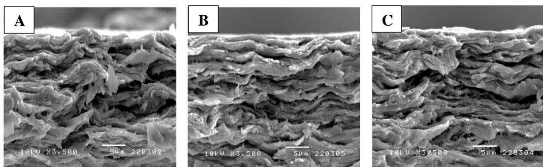
**Figure 4.31** SEM images of cross sectional morphology: the MBAGT films in dry state at concentration of 1%, 5% and 10% v/v mangosteen ethanolic extract
