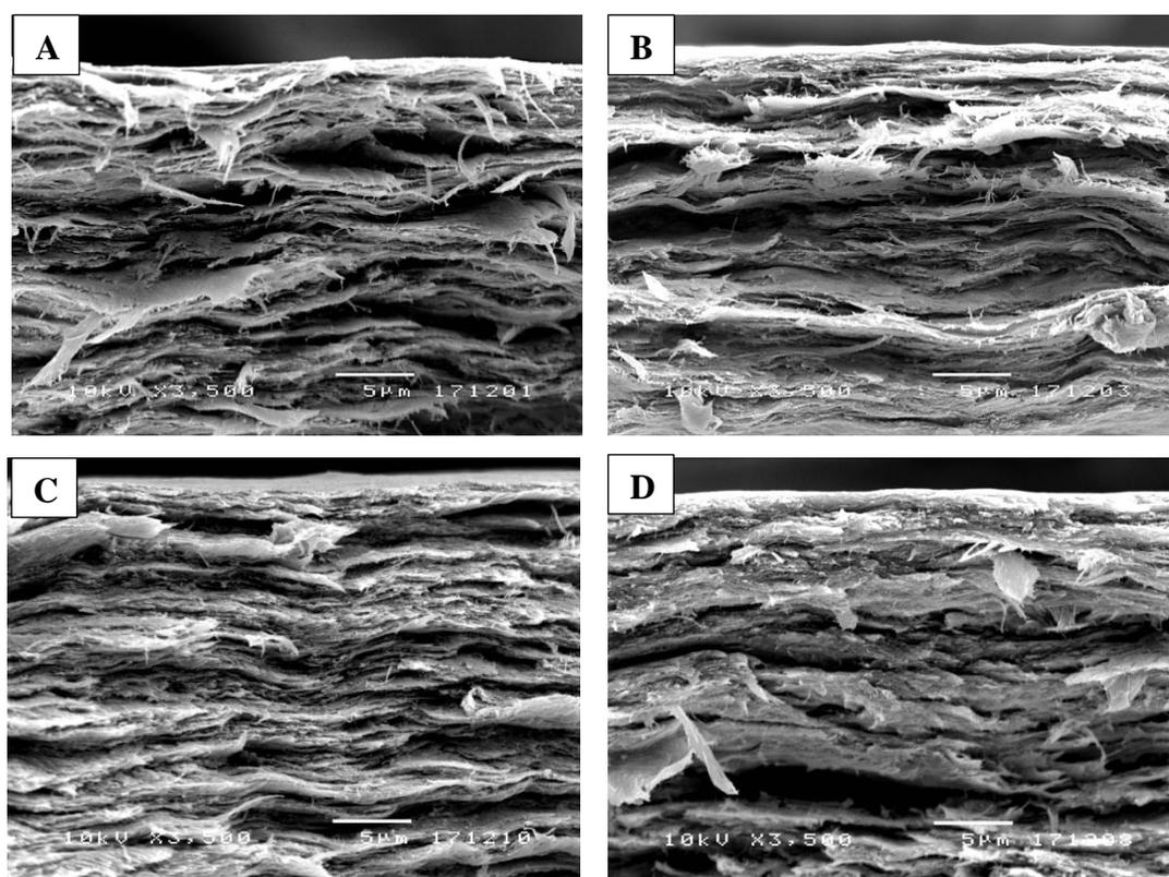
**Figure 4.13** SEM images of cross-sectional morphology: BAG films in dry form at a ratio of 60/10/30 (A), 60/20/20 (B), 60/30/10 (C) and MBAG film at 60/20/20 plasticized with glycerol (D)
