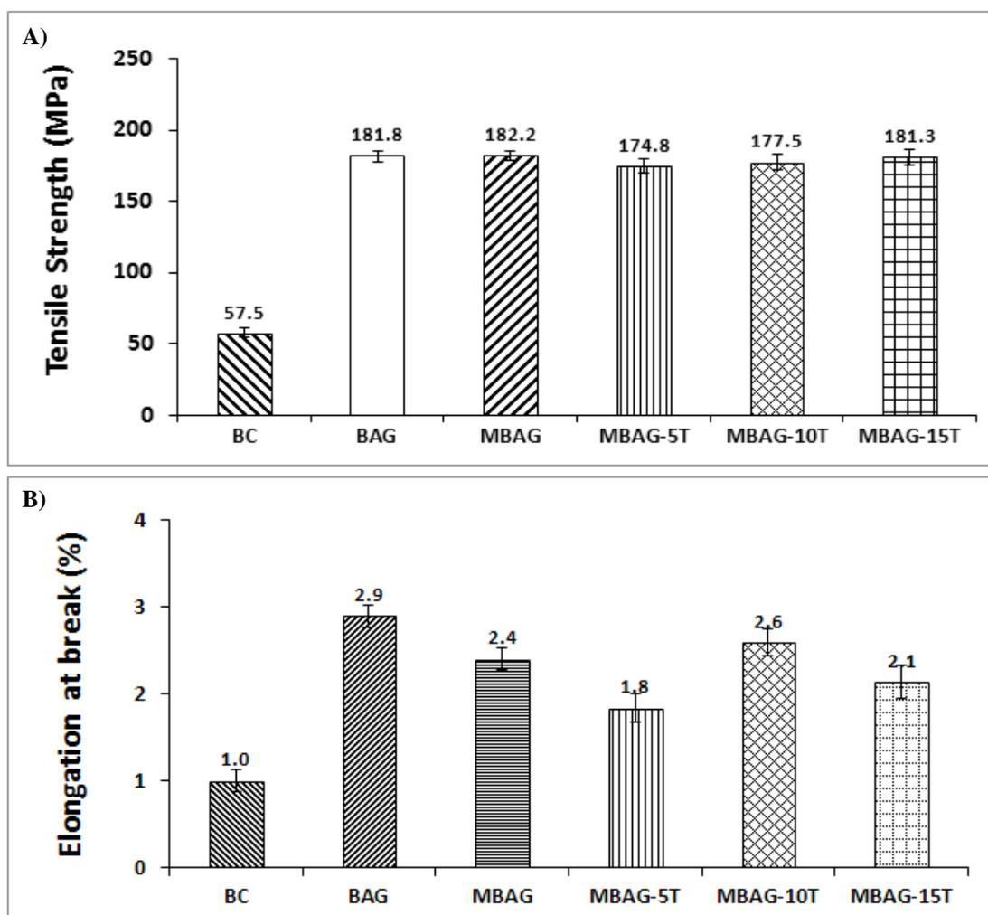
**Figure 4.17** Mechanical properties of BAG films in dry state at a ratio of 5, 10 and 15 mg tannic acid to g gelatin solution (w/w): Tensile strength (A) and Elongation at break (B).
