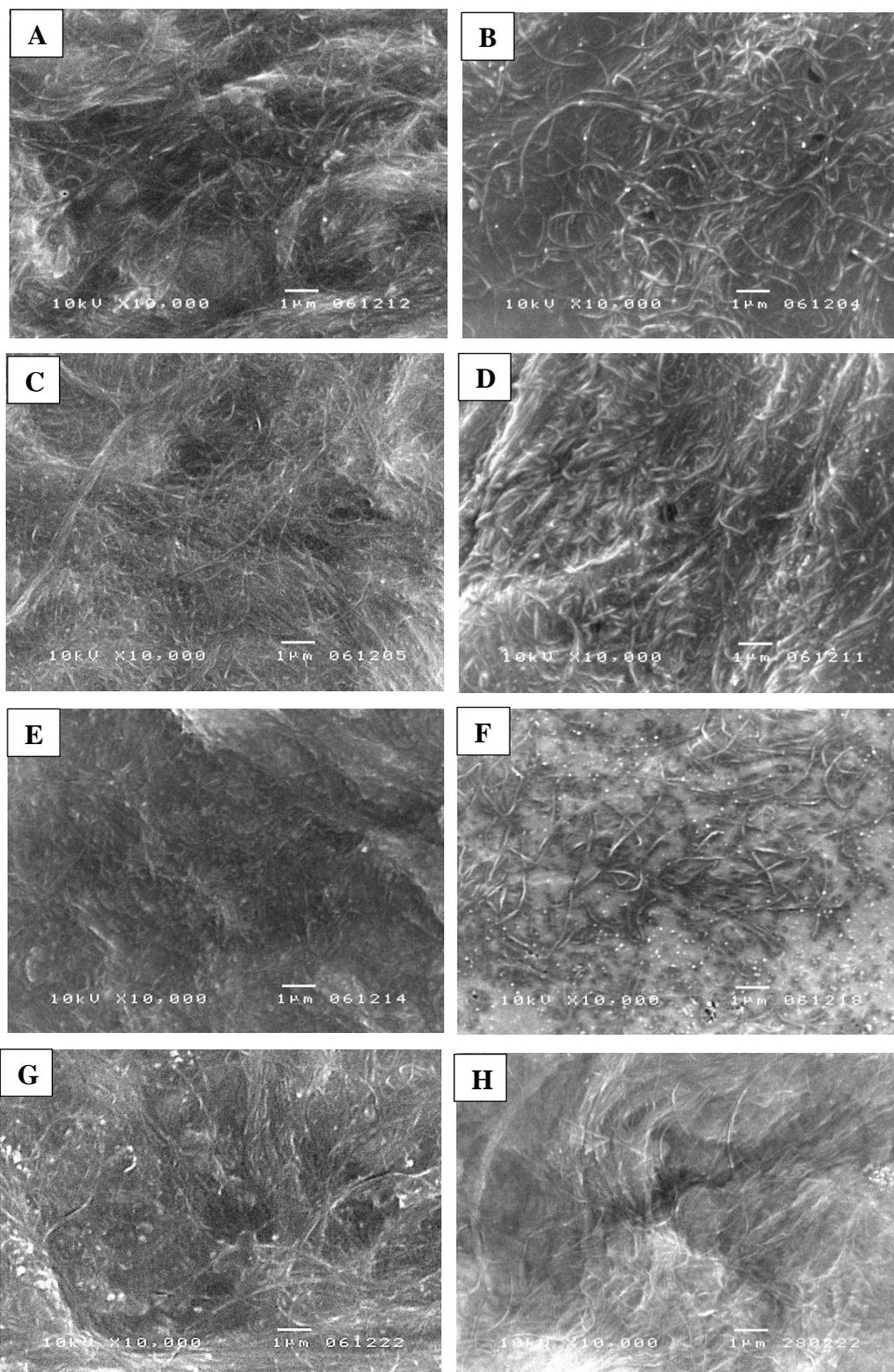
**Figure 4.12** SEM images of surface morphology of BAG films in dry (left) and re-swollen (right) forms at a ratio of 60/10/30 (A and B), 60/20/20 (C and D), 60/30/10 (E and F) and MBAG film at a ratio of 60/20/20 plasticized with glycerol (G and H)
