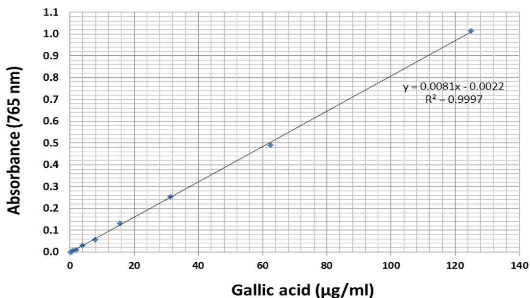
**Figure A1** Standard calibration curve of phenolic compound for quantitative determination of bioactive compounds content
