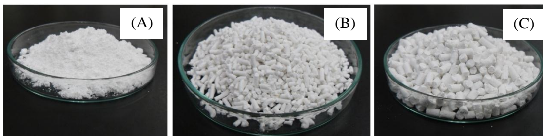
Figure 3.3 Photographs of the catalyst powdery ZSA-P (A) and extrudates ZSA-ME (B) and ZSA-SE (B).
