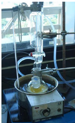
Figure 3.4 Experimental setup for the transesterification of palm oil with methanol under batch condition.
