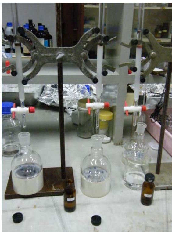
Figure 3.9 Fractionation process using silica gel chromatography column.
