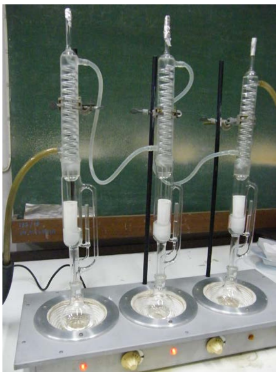
Figure 3.8 Soxhlet Extraction of coastal sediment samples.
