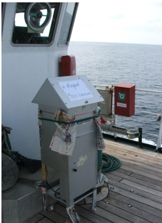
Figure 3.7 The high volume air sampler (Peak roof inlet) for collecting the ship-board aerosol.
