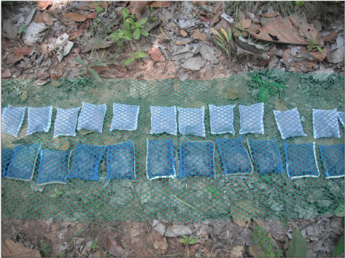
Figure 14 Litter bags, 0.5 mm mesh size (top row) and 2.0 mm mesh size (bottom row)
