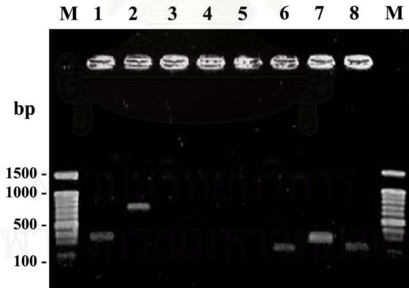
Figure 3.13 A 1.0% agarose gel electrophoresis showing colony PCR of PERT subtraction of genomic DNA of female (tester) and male (driver). Clones containing inserted DNA are found in lane 1 and 2. A 100 bp ladder was used as the DNA markers (lane M).
