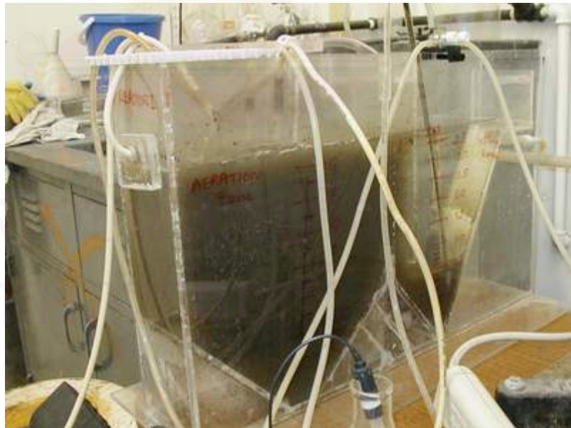
Figure 3.2 The bench-scale AS unit during normal operation
