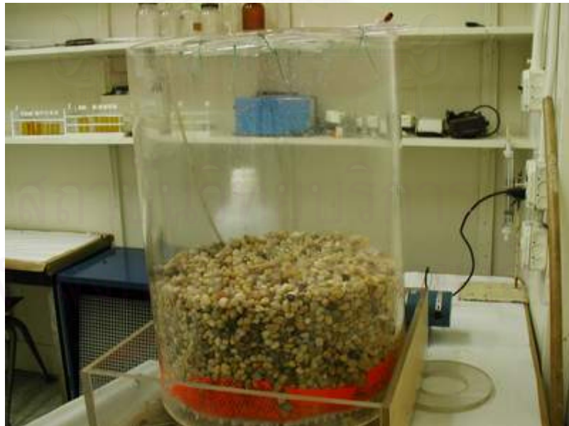
Figure 3.4 The bench-scale TF unit during normal operation
