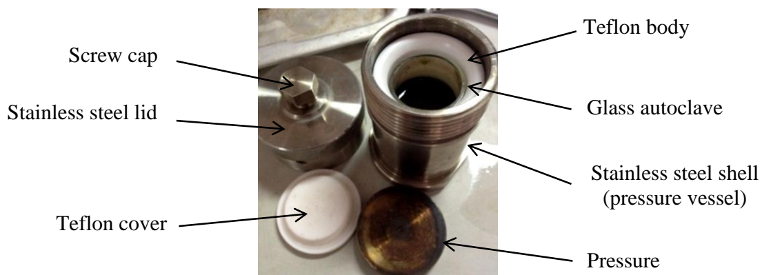
Figure 3.2 Small batch autoclave reactor
