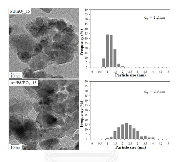
Figure 4.16 TEM images and distribution size of Pd/TiO $_2$ \_15 and Au/Pd/TiO $_2$ \_15
