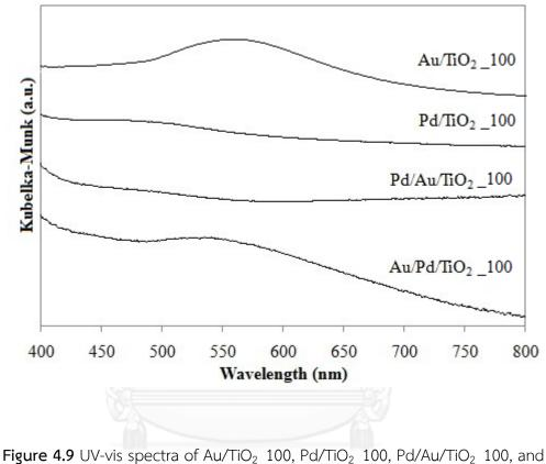
Figure 4.9 UV-vis spectra of Au/TiO<sub>2</sub>\_100, Pd/TiO<sub>2</sub>\_100, Pd/Au/TiO<sub>2</sub>\_100, and Au/Pd/TiO<sub>2</sub>\_100
