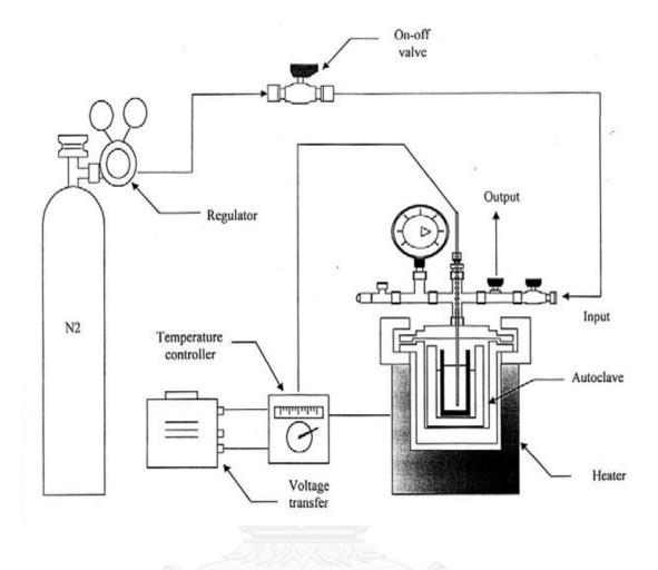
Figure 3.1 The schematic drawing of equipment used for the preparation of  $TiO_2$
