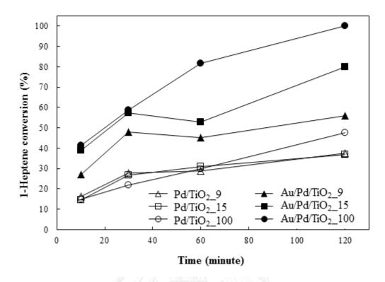
Figure 4.26 Hydrogenation of 1-heptene on Pd/TiO<sub>2</sub>\_9, Au/Pd/TiO<sub>2</sub>\_9, Pd/TiO<sub>2</sub>\_15, Au/Pd/TiO<sub>2</sub>\_15, Pd/TiO<sub>2</sub>\_100, and Au/Pd/TiO<sub>2</sub>\_100
