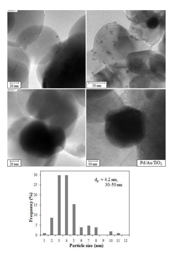
Figure 4.4 TEM images and particle size distribution of Pd/Au/TiO $_2$ \_100 catalyst
