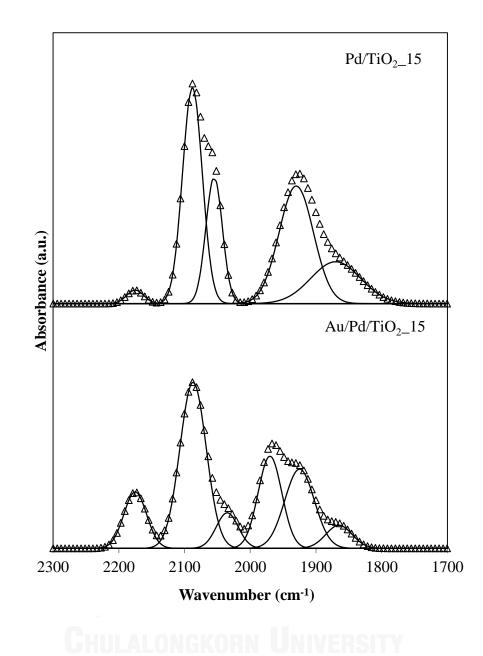
Figure 4.23 FTIR spectra of adsorbed CO at room temperature on Pd/TiO $_2$ \_15 and
