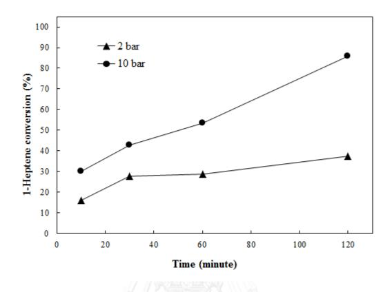
Figure 4.28 Hydrogenation of 1-heptene on Pd/TiO $_2_9$  catalyst under H $_2$  pressure of 2 and 10 bars
