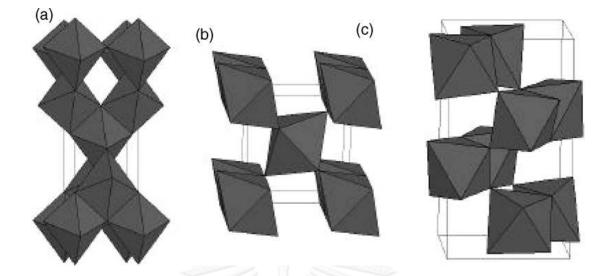
Figure 2.3 Crystal structures of anatase (a), rutile (b), and brookite (c) TiO<sub>2</sub>
