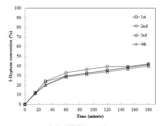
Figure 4.30 The catalyst deactivation test for hydrogenation of 1-heptene on
