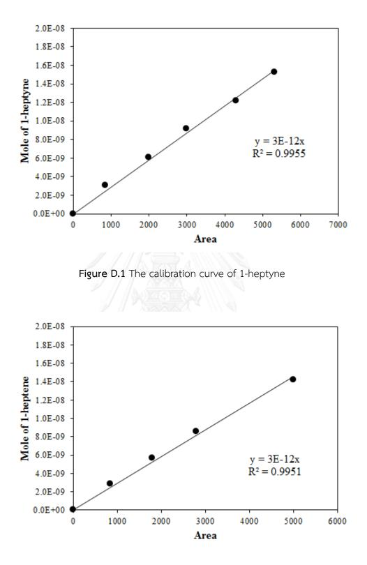
Figure D.2 The calibration curve of 1-heptene
