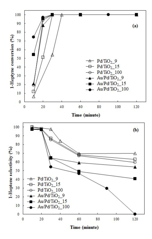
**Figure 4.25** Hydrogenation of 1-heptyne on Pd/TiO<sub>2</sub>\_9, Au/Pd/TiO<sub>2</sub>\_9, Pd/TiO<sub>2</sub>\_15, Au/Pd/TiO<sub>2</sub>\_15, Pd/TiO<sub>2</sub>\_100, and Au/Pd/TiO<sub>2</sub>\_100: %heptyne conversion (a) and %heptenes selectivity (b)
