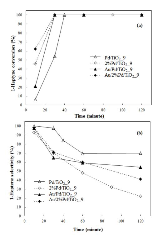
**Figure 4.27** Hydrogenation of 1-heptyne on Pd/TiO<sub>2</sub>\_9, 2%Pd/TiO<sub>2</sub>\_9, Au/Pd/TiO<sub>2</sub>\_9, and Au/2%Pd/TiO<sub>2</sub>\_9: % heptyne conversion (a) and % heptenes selectivity (b)
