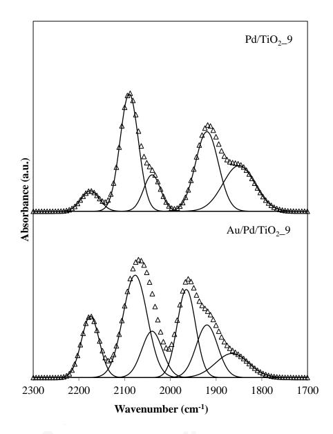
Figure 4.22 FTIR spectra of adsorbed CO at room temperature on Pd/TiO\_2\_9 and Au/Pd/TiO\_2\_9
