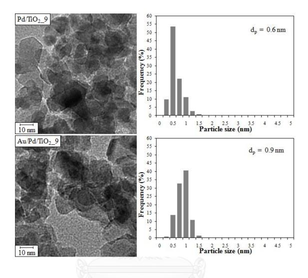
Figure 4.15 TEM images and distribution size of Pd/TiO<sub>2</sub>\_9 and Au/Pd/TiO<sub>2</sub>\_9
