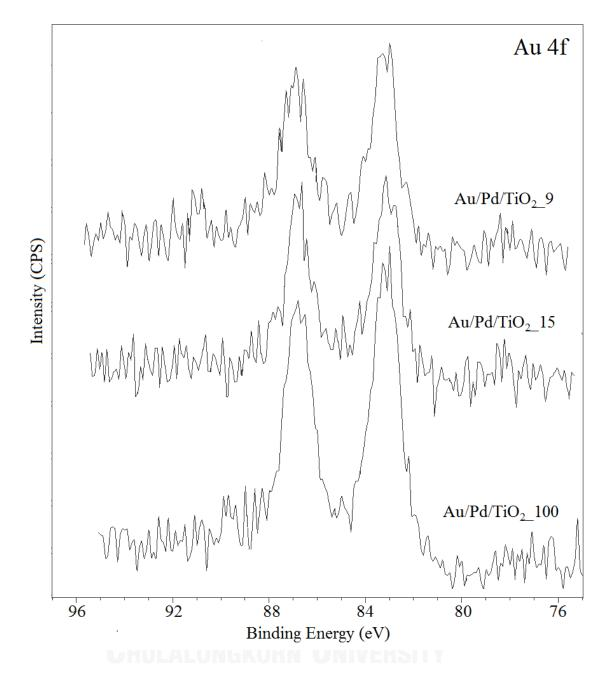
Figure 4.20 XPS Au 4f core level spectra of Au/Pd/TiO\_2\_9, Au/Pd/TiO\_2\_15, and Au/Pd/TiO\_2\_100
