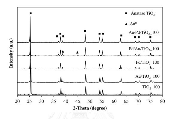
**Figure 4.1** XRD patterns of TiO<sub>2</sub>\_100, Au/TiO<sub>2</sub>\_100, Pd/TiO<sub>2</sub>\_100, Pd/Au/TiO<sub>2</sub>\_100, and Au/Pd/TiO<sub>2</sub>\_100 catalysts
