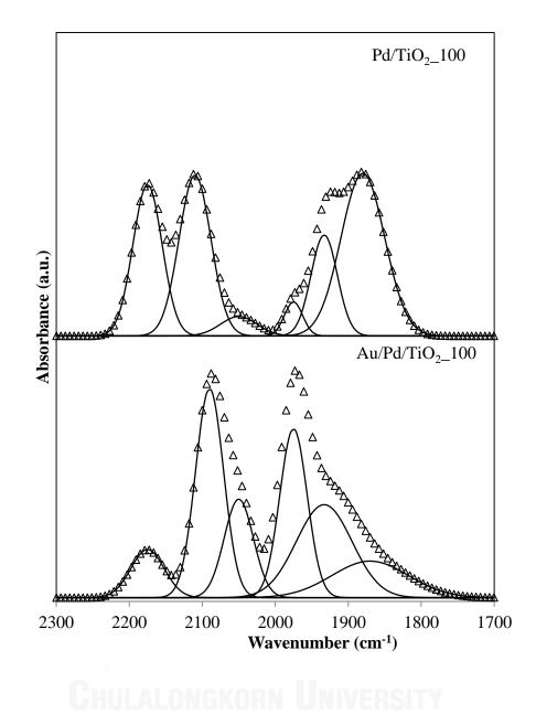
Figure 4.24 FTIR spectra of adsorbed CO at room temperature on Pd/TiO\_2\_100 and Au/Pd/TiO\_2\_100
