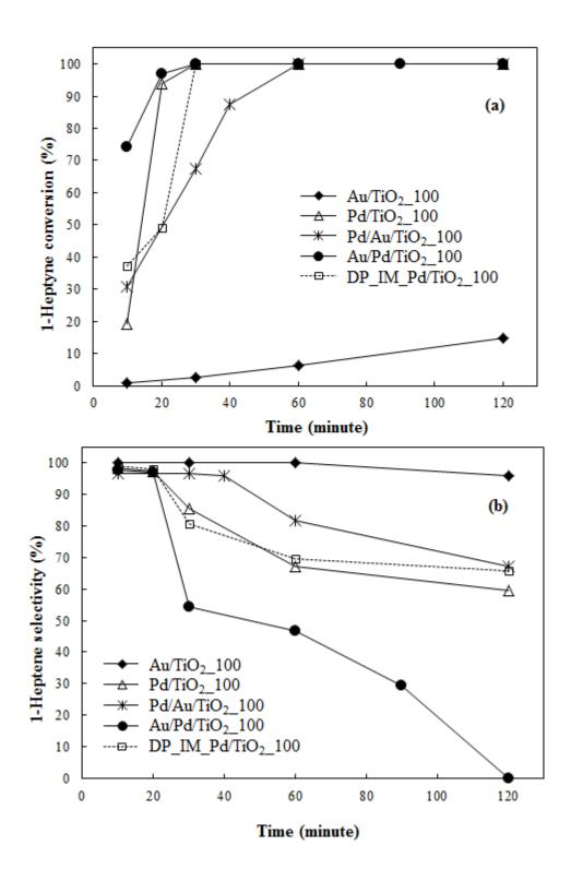
**Figure 4.11** Hydrogenation of 1-heptyne on Pd/TiO<sub>2</sub>\_100, Pd/Au/TiO<sub>2</sub>\_100, and Au/Pd/TiO<sub>2</sub>\_100: %heptyne conversion (a) and %1-heptene selectivity (b)
