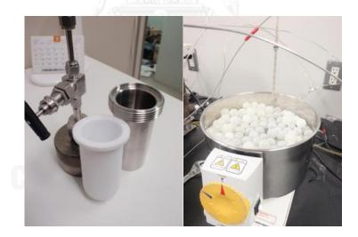
Figure 3.3 Teflon-lined stainless steel autoclave reactor of liquid-phase hydrogenation
