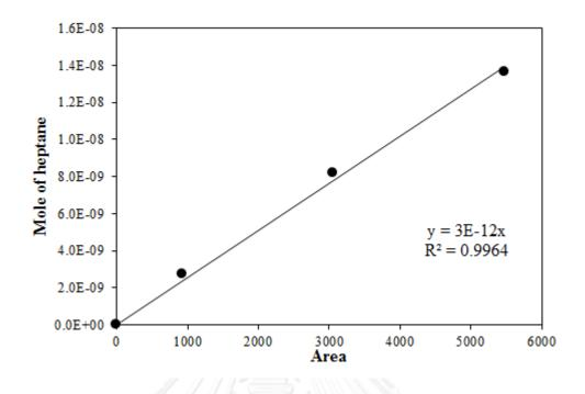
Figure D.3 The calibration curve of heptane
