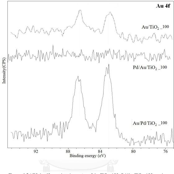
Figure 4.8 XPS Au 4f core level spectra of Au/TiO\_100, Pd/Au/TiO\_100, and Au/Pd/TiO\_100
