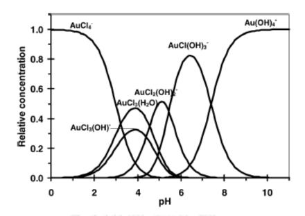
Figure 2.2 Relative equilibrium concentration of gold complexes ( $[Cl]^{-} = 2.5 \times 10^{-3} \text{ M}$ ) as a function of the pH of the solution, calculated with equilibrium constants reported by Nechayev et al.
