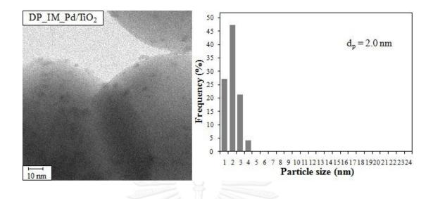
Figure 4.6 TEM images and particle size distribution of  $DP_IM_Pd/TiO_2_100$  catalyst
