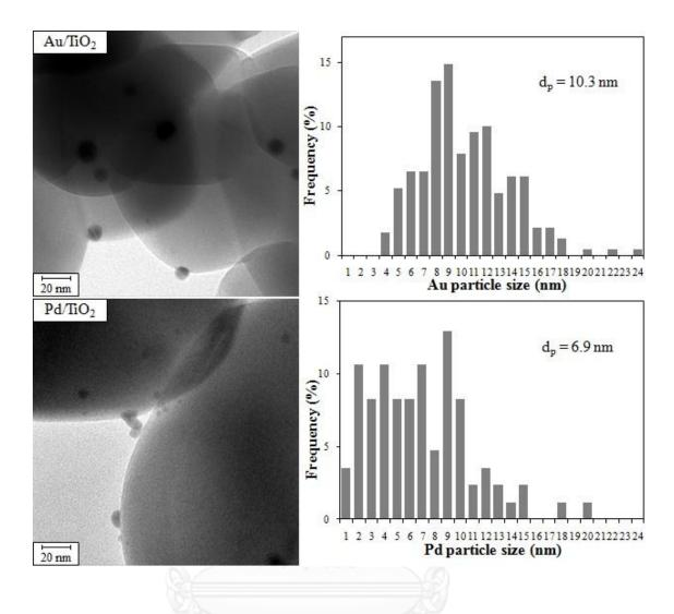
Figure 4.3 TEM images and particle size distribution of  $TiO_2$  supported Au and Pd
