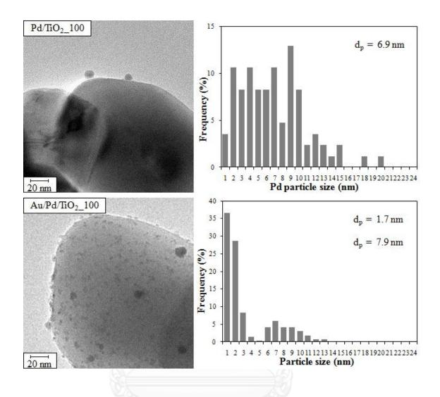
Figure 4.17 TEM images and distribution size of  $Pd/TiO_2_100$  and  $Au/Pd/TiO_2_100$
