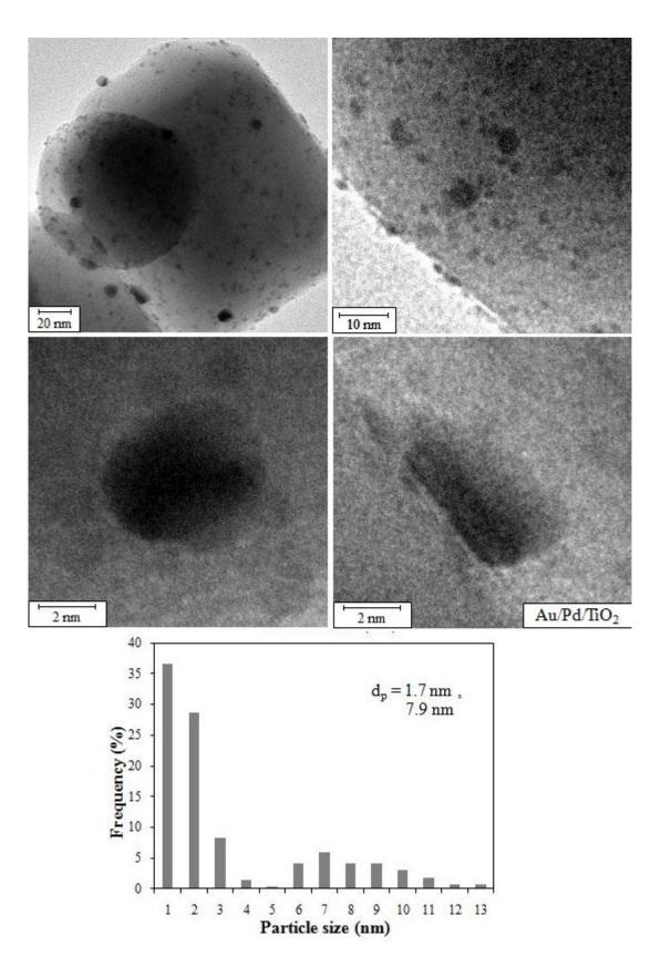
Figure 4.5 TEM images and particle size distribution of Au/Pd/TiO<sub>2</sub>\_100 catalyst
