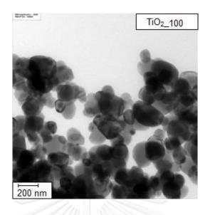
Figure 4.2 TEM image of TiO<sub>2</sub>\_100 support
