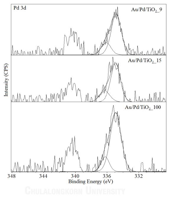
Figure 4.19 XPS Pd 3d core level spectra of Au/Pd/TiO\_2\_9, Au/Pd/TiO\_2\_15, and Au/Pd/TiO\_2\_100
