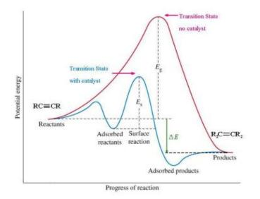
Figure 2.1 Potential energy profiles for non-catalysed and catalysed reactions
