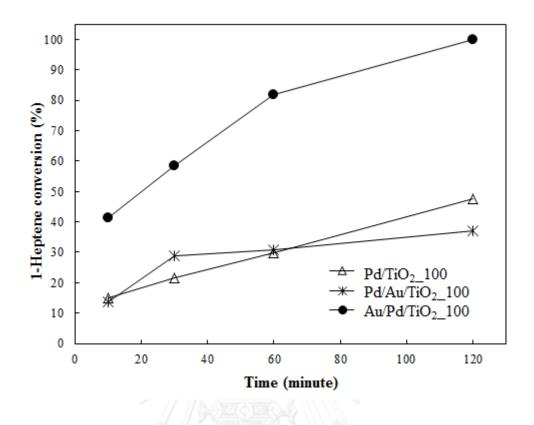
Figure 4.13 Hydrogenation of 1-heptene on Pd/TiO<sub>2</sub>\_100, Pd/Au/TiO<sub>2</sub>\_100, and
