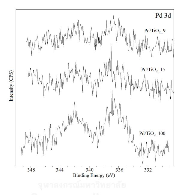
Figure 4.18 XPS Pd 3d core level spectra of Pd/TiO2\_9, Pd/TiO2\_15, and Pd/TiO2\_100
