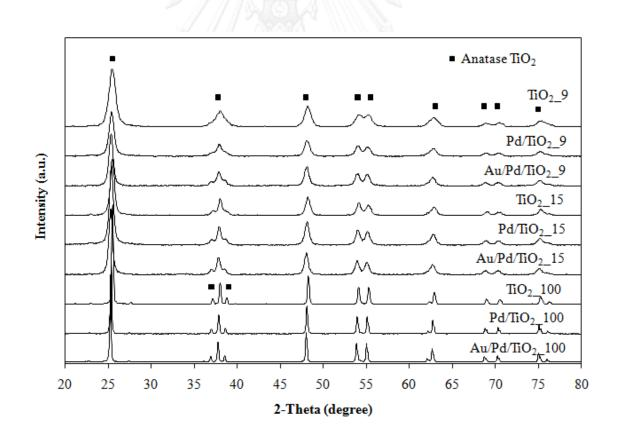
Figure 4.14 XRD patterns of TiO<sub>2</sub>\_9, Pd/TiO<sub>2</sub>\_9, Au/Pd/TiO<sub>2</sub>\_9, TiO<sub>2</sub>\_15, Pd/TiO<sub>2</sub>\_15, Au/Pd/TiO<sub>2</sub>\_15, TiO<sub>2</sub>\_100, Pd/TiO<sub>2</sub>\_100, and Au/Pd/TiO<sub>2</sub>\_100
