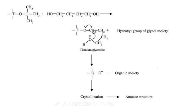
Figure 2.4 Mechanism of solvothermal reaction for the anatase  $TiO_2$  formation
