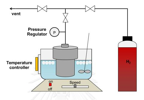
Figure 3.2 The schematic diagram of liquid-phase hydrogenation
