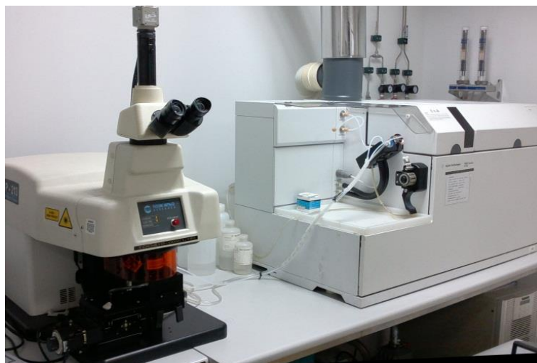
Figure 1.7 Laser Ablation-Inductivity Coupled Plasma-Mass Spectrometer (LA-ICP-MS), an Agilent, Model 7500 series based at the GIT.
