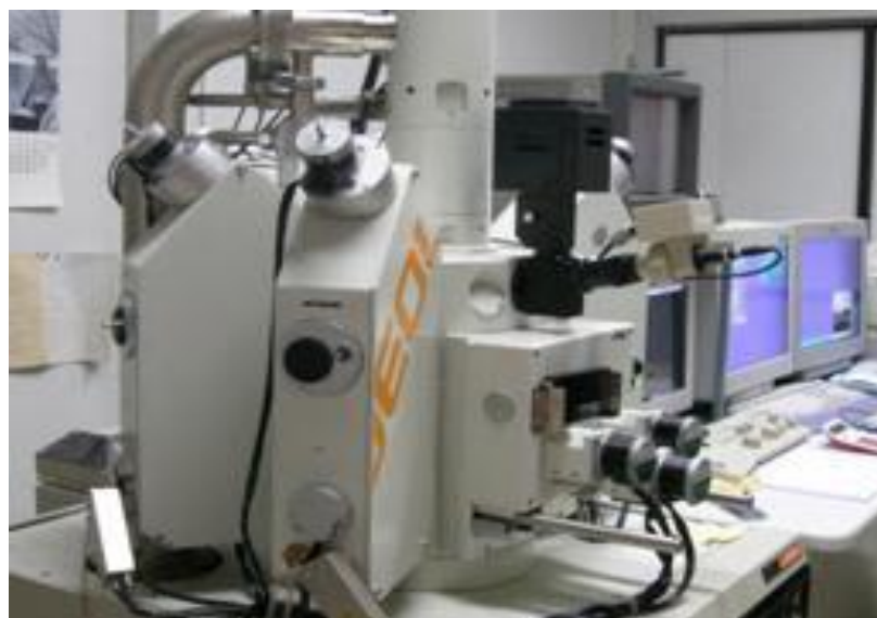
Figure 1.6 Electron Probe Micro – Analyzer (EPMA), Model JXA-8100 super probe, JEOL based at the Department of Geology, Faculty of Science, Chulalongkorn University.
