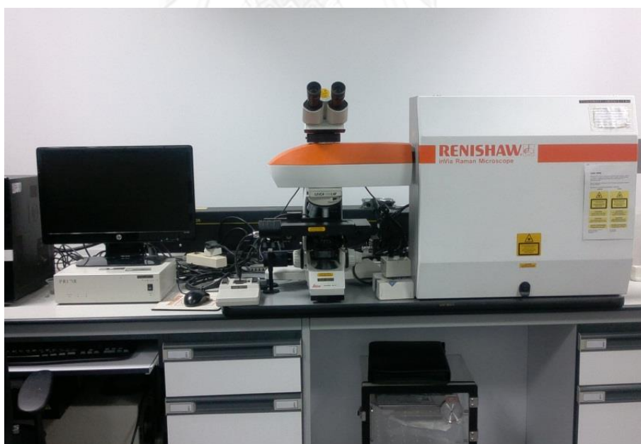
Figure 1.3 Laser Raman spectroscopy, Model Renishaw inVia Raman Microscope based at the GIT.
