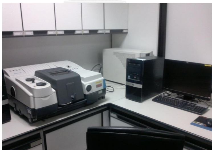
Figure 1.4 Fourier Transform Infra-Red (FTIR) spectrophotometer, Nicolet NEXUS 670 series based at the GIT.
