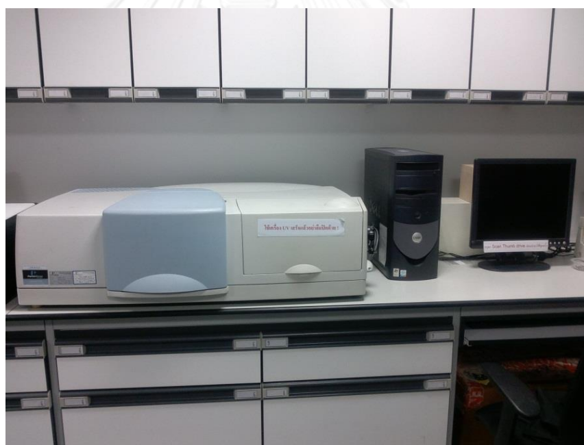
Figure 1.2 UV-VIS-NIR spectrophotometer, Model Lambda 950 series, Perkin Elmer based at the GIT.
