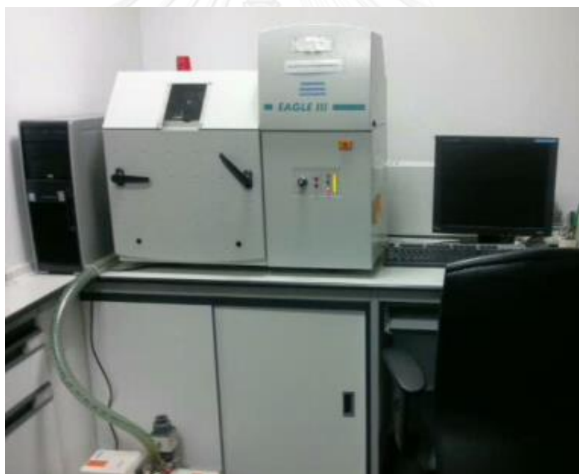
Figure 1.5 Energy Dispersive X-ray Fluorescence Spectrometer (EDXRF), Model Eagle III microprobe series, EDAX based at the GIT.
