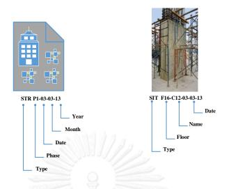
Figure 4.16 File name of BIM-record model for a column
