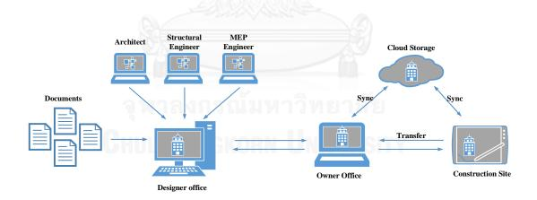
Figure 4.4 System architecture of BIM-based construction project monitoring system
