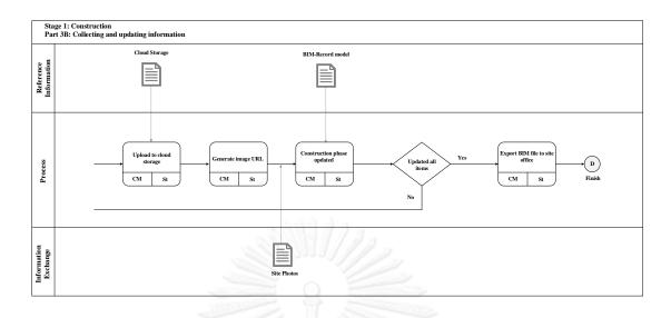
Figure 4.14 Workflow of the data collection and project updating part
