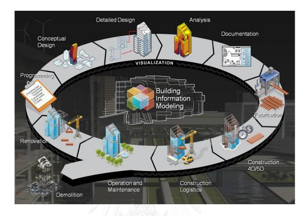
Figure 2.2 BIM-Building life cycle (Source: http://www.arquibim.es)
