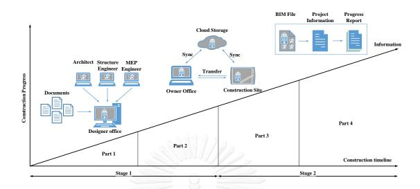
Figure 4.7 Stages and parts of the proposed system
