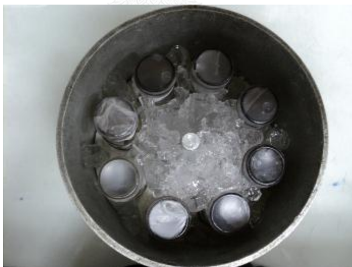
Figure 3.4 Ice cubes in water around the container for irradiation
