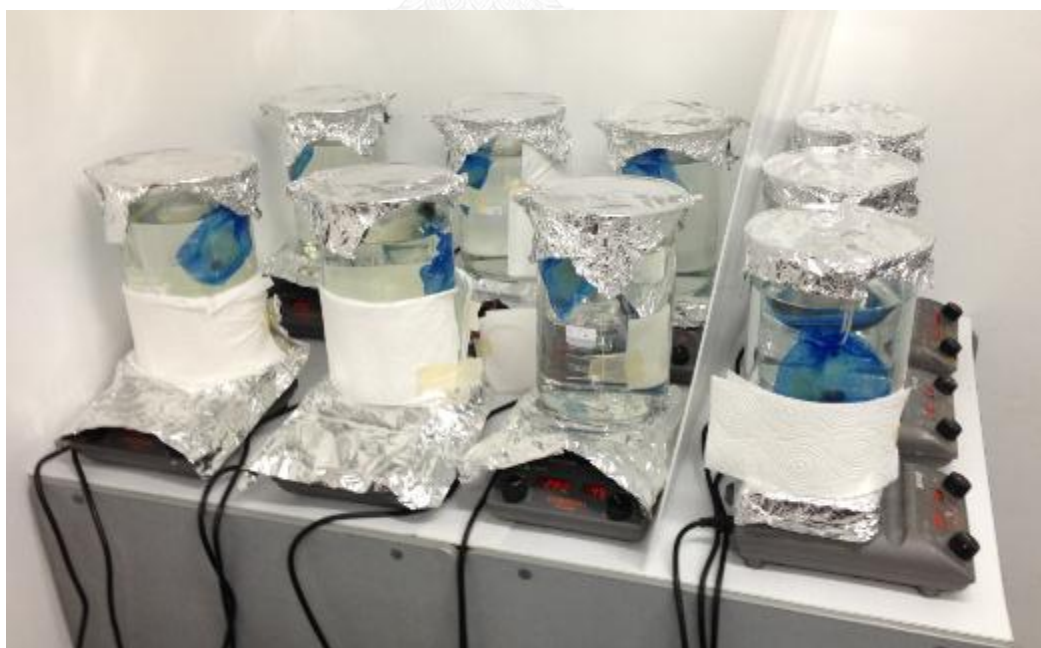
Figure 3.19 Experiment on the effect of pH and temperature on uranium extraction from seawater using non-chromic acid pre-treated amidoxime fibers
