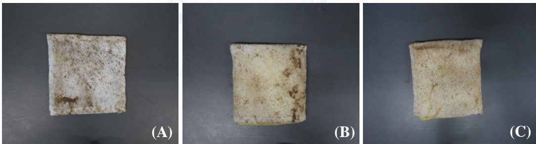
Figure 4.7 Decomposing polyester during rainy season after 2 weeks (A), 4 weeks (B), 6 weeks (C)
