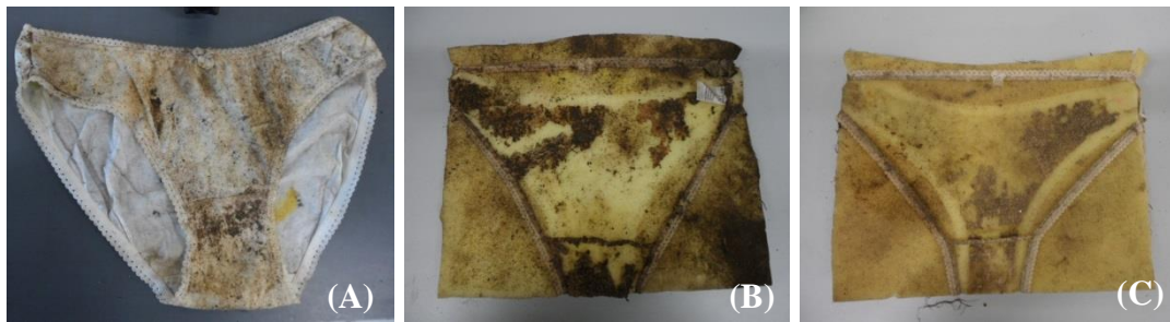
Figure 4.5 Decomposing briefs during rainy season after 2 weeks (A), 4 weeks (B), 6 weeks (C)
