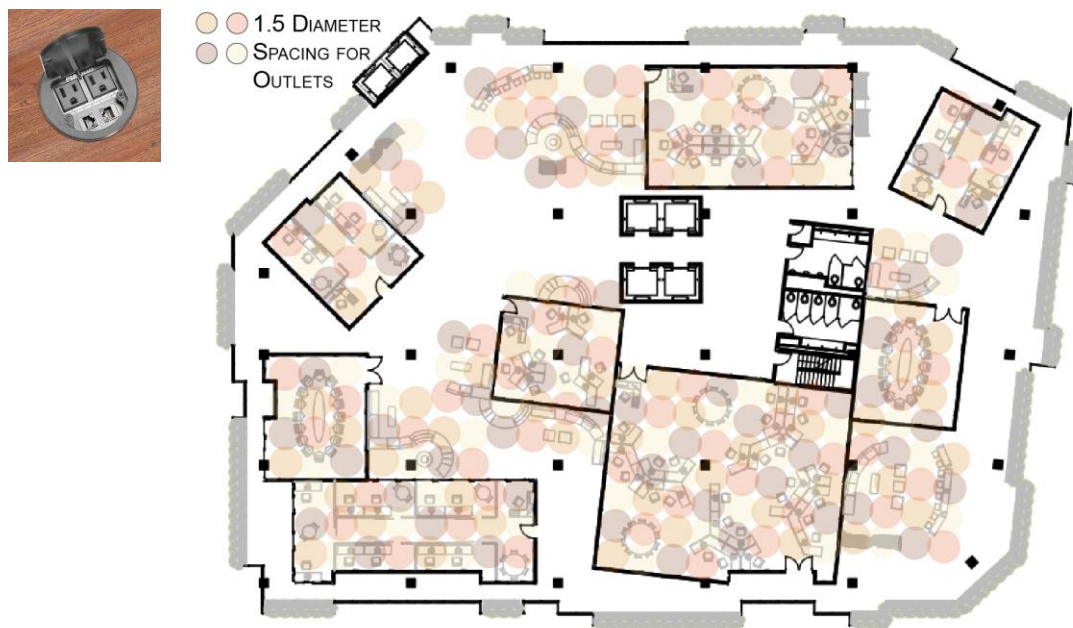
Figure 7. 5 Outlet Array Example Level 4, 7, & 10 Building 3
