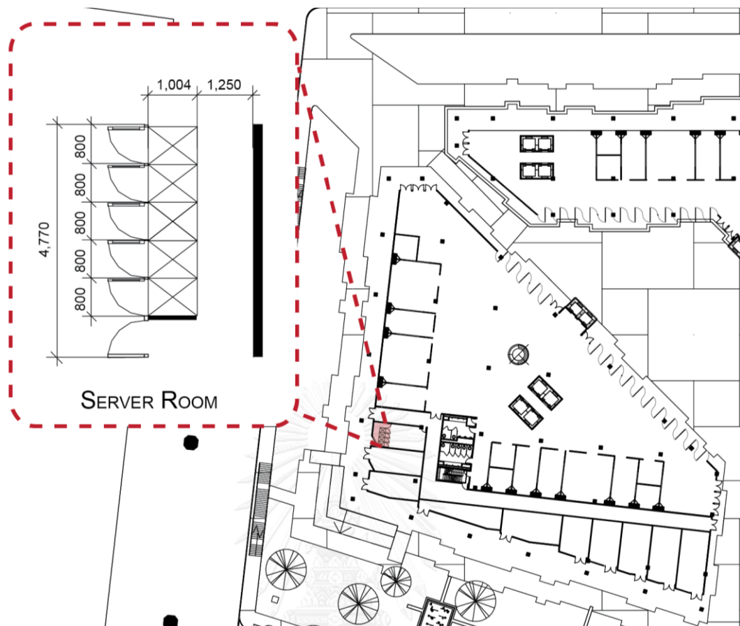
Figure 7. 3 Server Room Building 1
