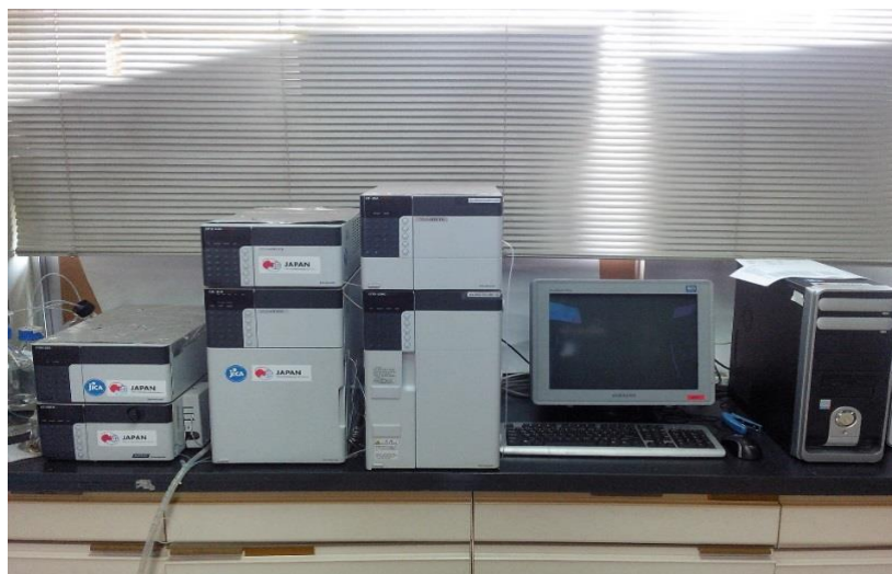
Figure A.7 High Performance Liquid Chromatography (HPLC) Fluorescence detector and UV detector
