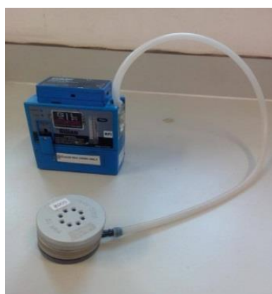
Figure A.3 Personal air pump connected to personal modular impactor (PMI)
